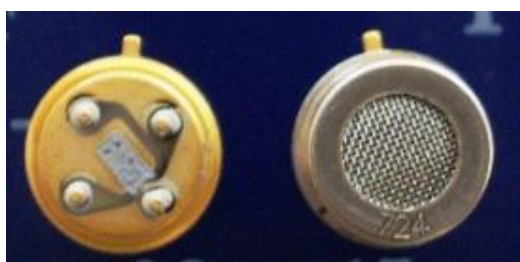
Figure III.2: Synkera 725 sensor response [28] Figure III.3: Synkera 725 MOX sensor[28]
