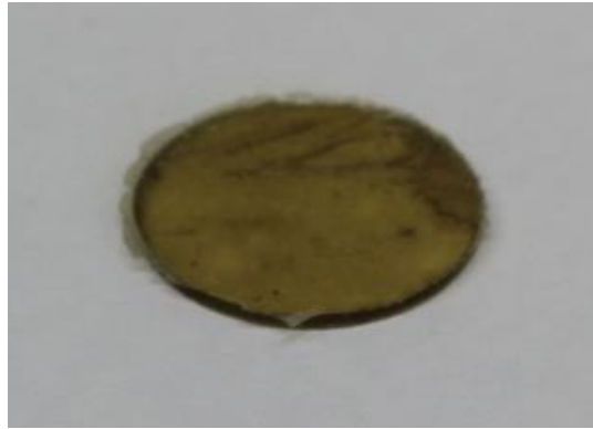
Figure 36. Macroscopic Photo PEI 1% fill by weight 80 mesh.
