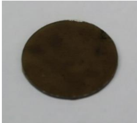
Figure 12. Photograph of press melted PEI Specimen.
