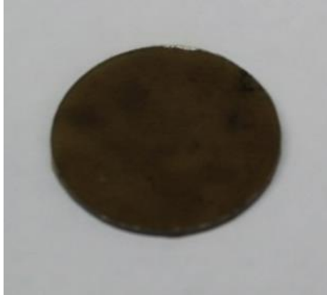
Figure 32. Macroscopic Photo PEI 1% fill by weight 40 mesh.
