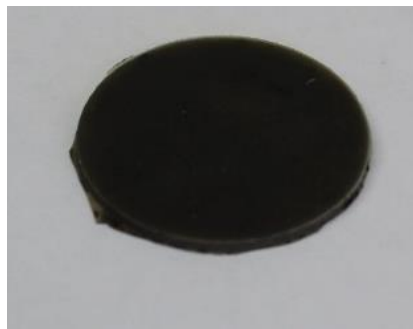
Figure 33. Macroscopic Photo PEI 5% fill by weight 40 mesh.
