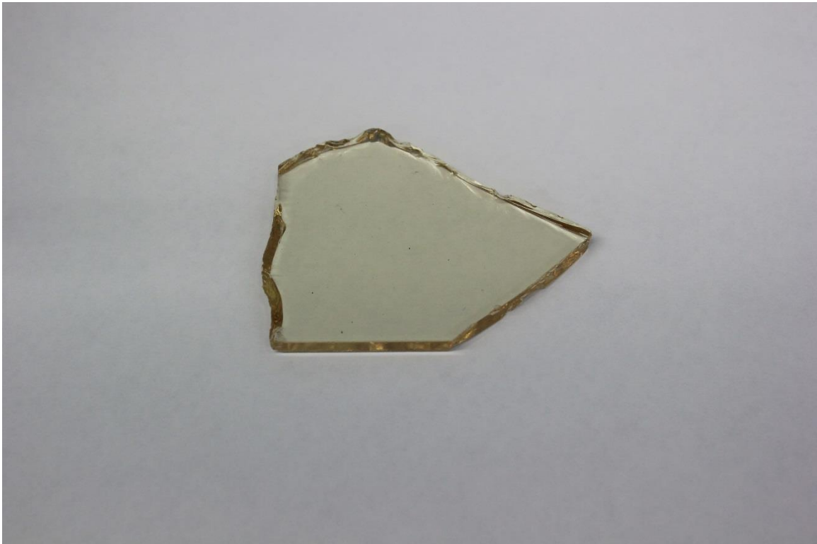
Figure 8. Bulk Nextrema 2.63 cm in the longest direction.
