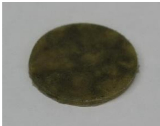
Figure 37. Macroscopic Photo PEI 5% fill by weight 80 mesh.
