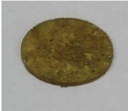
Figure 34. Macroscopic Photo PEI 1% fill by weight 40-80 mesh.
