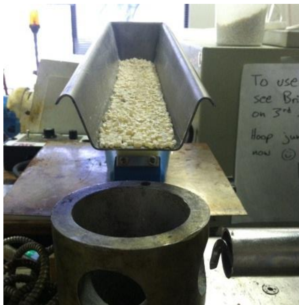
Figure 9. PEI/Nextrema particles fed into the extruder by the vibrating feeder trough.
