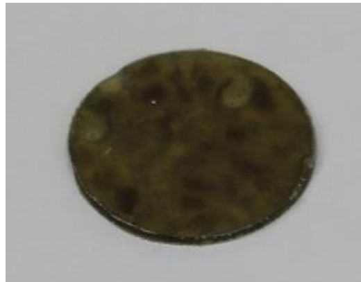
Figure 35. Macroscopic Photo PEI 5% fill by weight 40-80 mesh.
