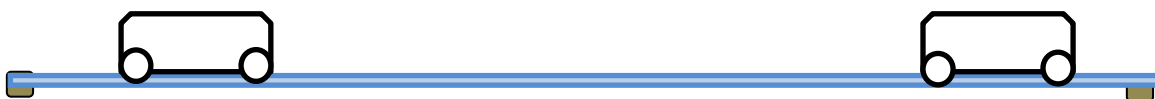
Figure 5. Two carts on a grooved track, with their magnetic ends facing each other.
