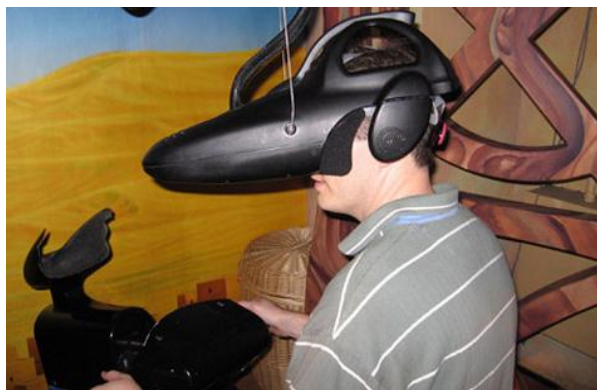
Figure 2.7: Adjustable HMD Liner with HMD (Disney Quest 2012)
