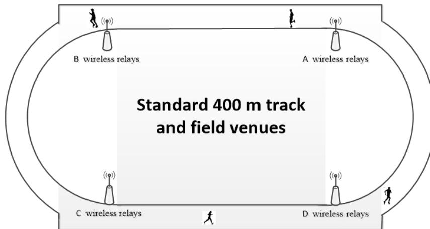
Figure 2. The location of the heart rate wireless receiver in a standard athletic field
