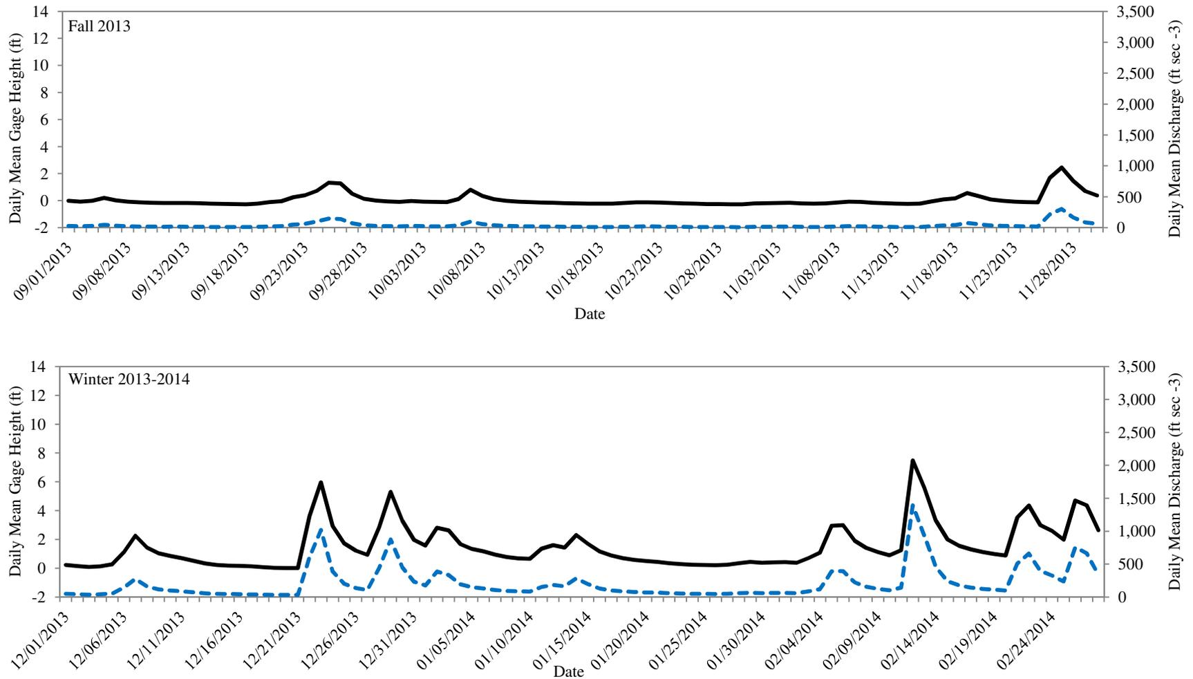
Figure 3.10 (continued). Daily mean gage height (ft; solid line) on the primary y-axis and daily mean discharge (ft sec<sup>-3</sup>; dashed line) on the secondary y-axis for the Biloxi River at the Wortham, MS (U.S.G.S monitoring station 02481000; <http://waterdata.usgs.gov>) which is located approximated 12 river km above the study area.
