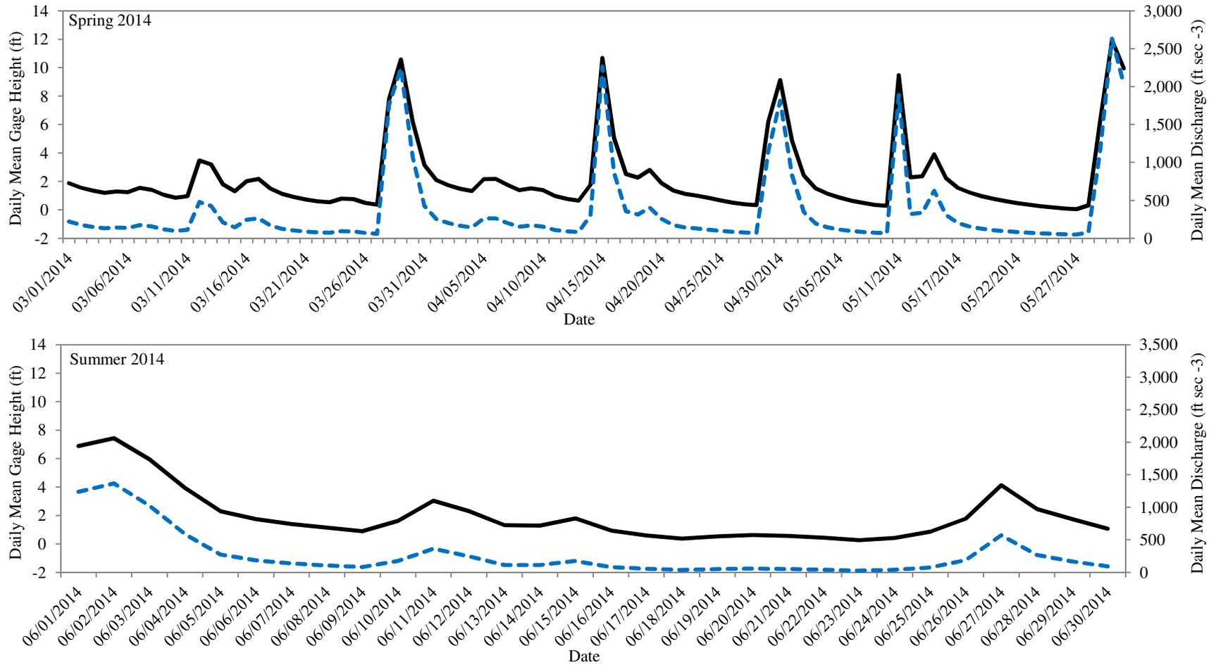
Figure 3.10 (continued). Daily mean gage height (ft; solid line) on the primary y-axis and daily mean discharge (ft sec<sup>-3</sup>; dashed line) on the secondary y-axis for the Biloxi River at the Wortham, MS (U.S.G.S monitoring station 02481000; <http://waterdata.usgs.gov>), which is located approximated 12 river km above the study area.
