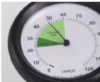
Intra-cuff pressures can be measured by anesthesia providers with a quick and inexpensive device utilizing the practice of manometry monitoring. The manometer fits on the end of the LMA airway device in the pilot balloon to read the pressure number.
