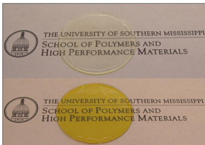
Figure A4. Photograph illustrating the ability to spin coat the liquid resins into thin films prior to sequential UV and thermal cure. The UV cure was carried out at room temperature for 20 min ( 365 \text{ nm} , 36 \text{ mW/cm}^2 ). The thermal cure was carried out at 180 \text{ }^\circ\text{C} in an air circulated oven for 3 h. The resin darkens towards a brownish-red color with increasing temperature.
