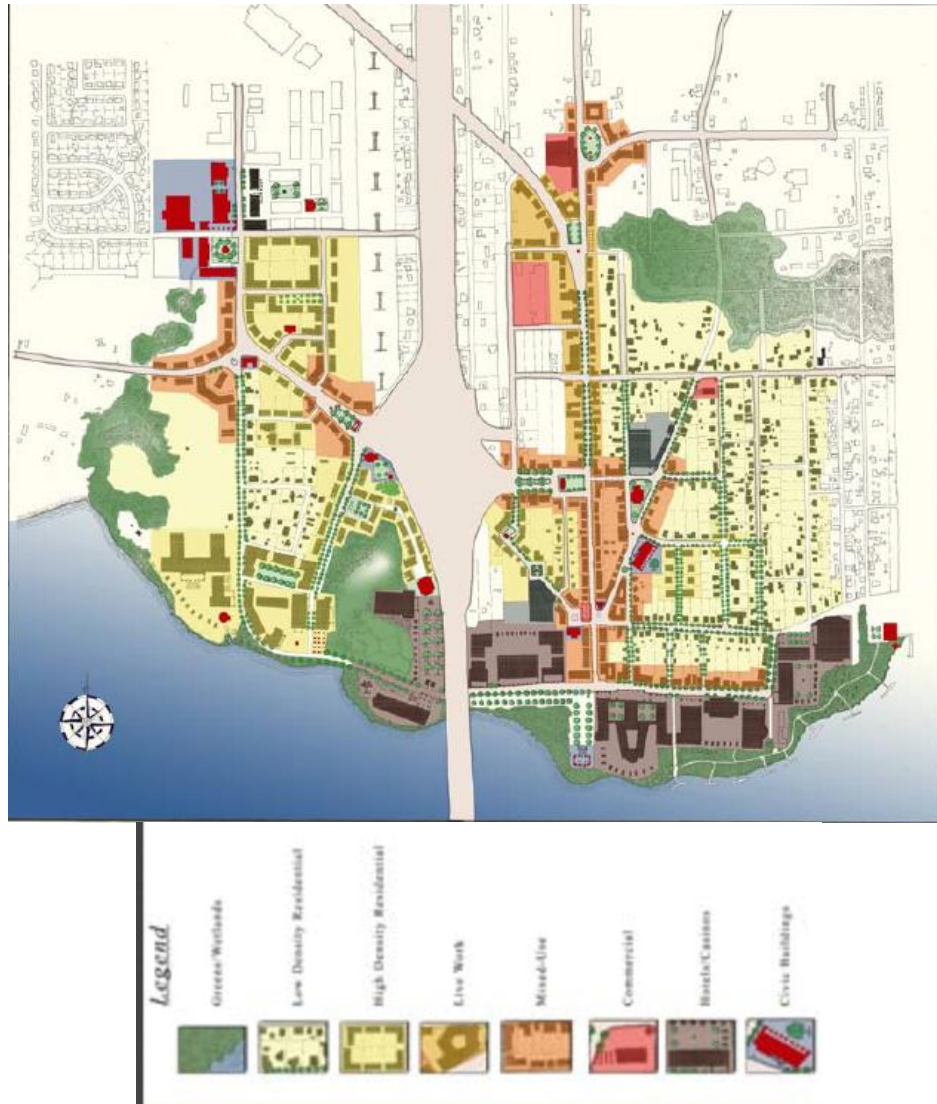
Figure 4- The Master Concept Plan of D'Iberville, Mississippi. The hotel/casinos are located along the waterfront. The light yellow parcels and dark yellow parcels are LDR and HDR. The blue and red parcels are civic buildings.
