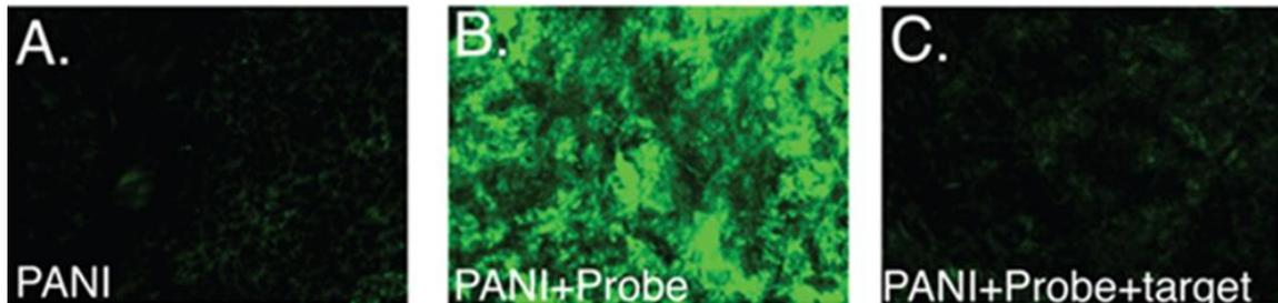
**Figure 5.** A. PANI Fluorescence emission is low B. PANI+Probe produces a significant amount of fluorescence C. PANI+Probe+target shows that basal fluorescence was achieved due to dissociation of hybridized duplex
