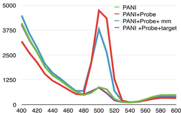
**Figure 6.** Fluorescence emission at optimum wavelength; PANI and PANI+Probe+target show low levels of fluorescence. The PANI+Probe+mismatch has high fluorescence still, showing the specificity of the sensor
