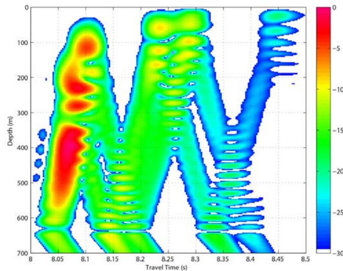
**Figure 12: This figure shows the arrival wave front for a forward simulation.** This wave front was formed from a source that was 150m deep; the final wavefront was then used with the edited wave time reversal code to obtain a similar plot:
