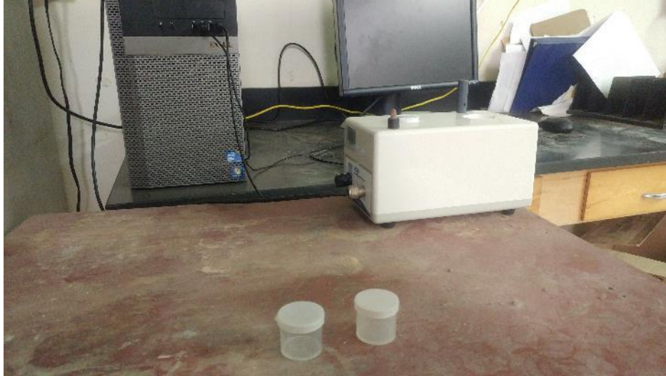
Figure 10: Image of the MS2B susceptibility unit, plastic vials, and desktop computer used in the magnetic susceptibility measurements.
