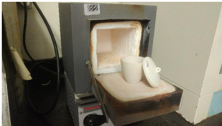
Figure 11: Image of muffle furnace and crucibles used in the loss-on ignition test.
