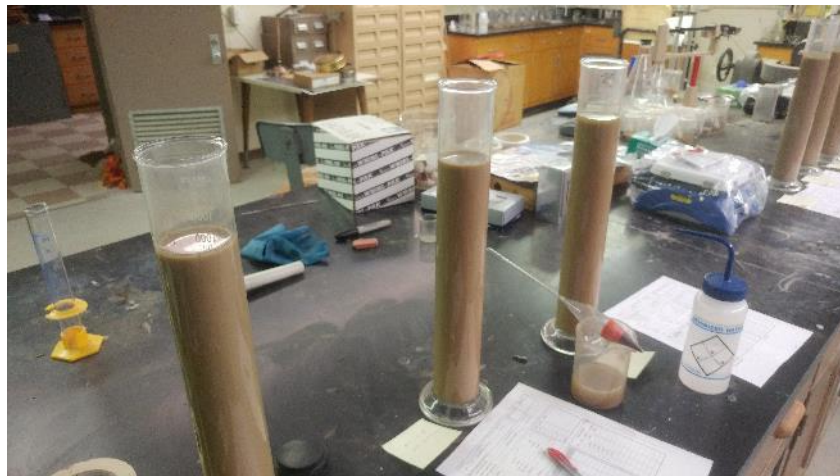
Figure 12: Image of Bouyoucos tubes and a hydrometer being used in sediment size analyses.
