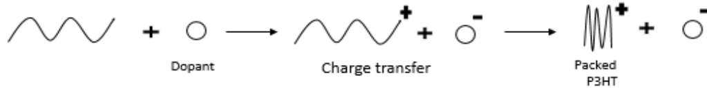
Figure 1 - Possible mechanism for doping 1: Charge transfer occurs before aggregation
