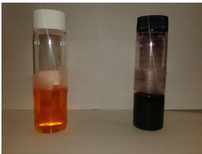
Figure 4 - (left) solubilized P3HT; (right) aggregated P3HT
