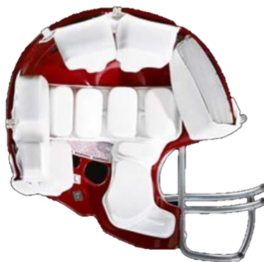
Figure 2 was pulled from the study of Gale A et al , performed in 1985 and shows an American football helmet with the outer polycarbonate shell component shown in red and the inner lining of the pads and foams shown in white.
