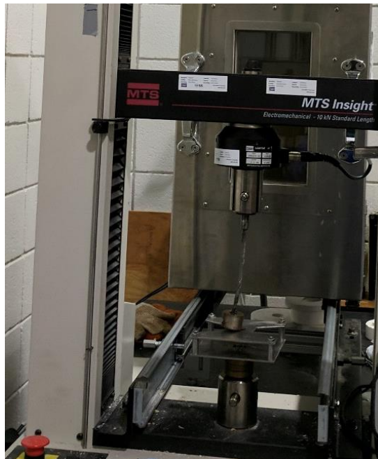
Figure 6: MTS Pull-Off Adhesion Load Frame.
