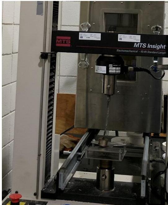
Figure 6: MTS Pull-Off Adhesion Load Frame.
