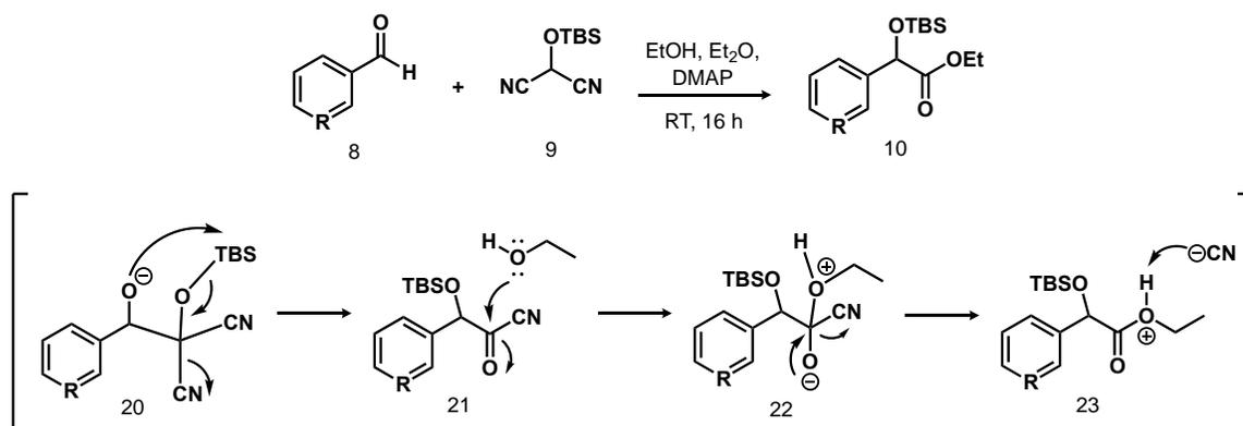
*Scheme 4.3: Generalized reaction scheme and proposed mechanism*
