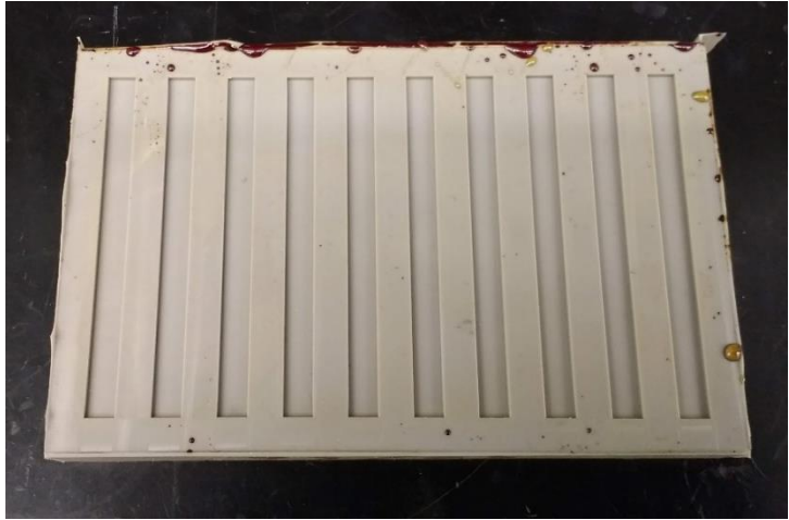
Figure 1 Typical silicon DMA mold used to cure epoxy-amine samples.
