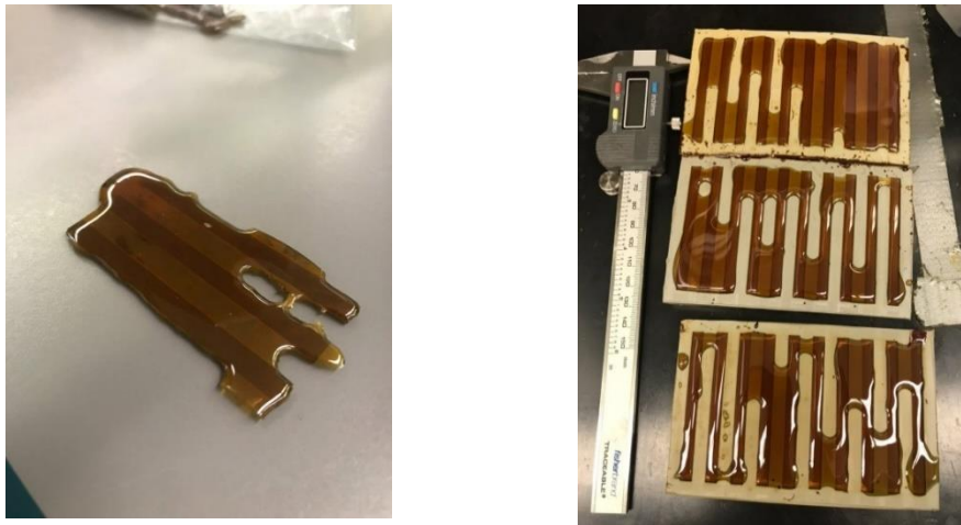
Figure 3 (Left) 3 Unsanded DMA bars that have been taken out of the DMA mold. (Right) 3 sets of DMA molds that have fully cured samples.
