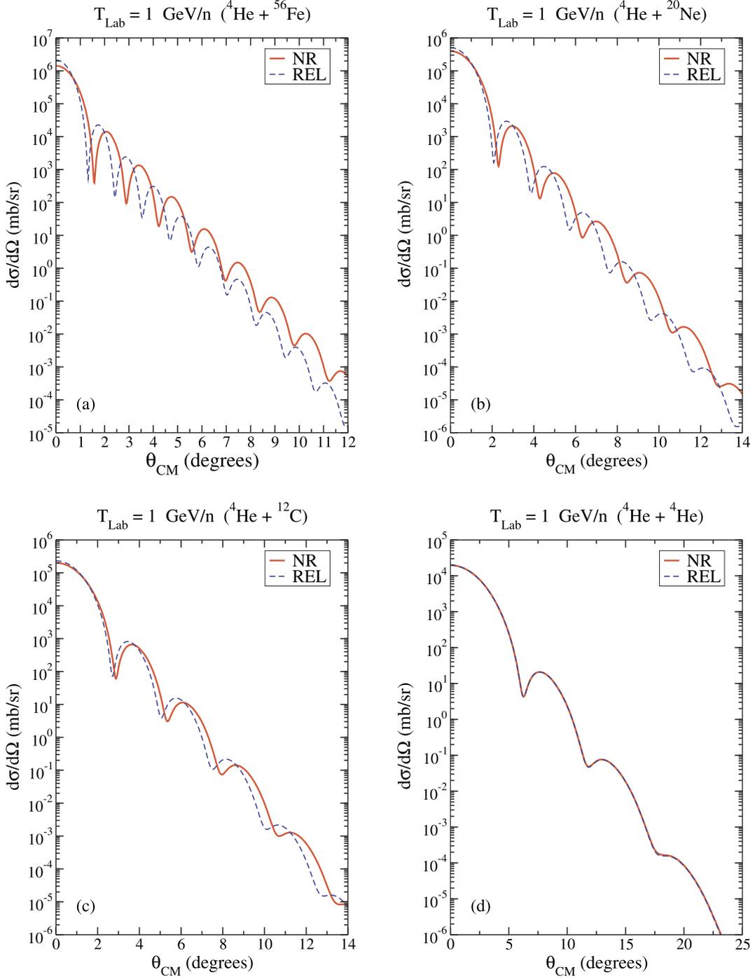
**Fig. 1.** Elastic differential cross sections for  ${}^4\text{He} + {}^{56}\text{Fe}$ ,  ${}^4\text{He} + {}^{20}\text{Ne}$ ,  ${}^4\text{He} + {}^{12}\text{C}$ , and  ${}^4\text{He} + {}^4\text{He}$  reactions at a lab projectile energy of 1 GeV/n. NR results are indicated with solid red lines, and REL results are given as dashed blue lines. (For interpretation of the references to color in this figure legend, the reader is referred to the web version of this article.)
