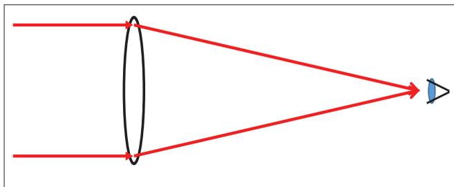
Fig. 2. Parallel rays converge to the focal point after passing through a convex lens. The distance from the lens to the focal point is the focal length of the lens. The result is that the observer sees a focused image.
