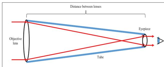
Fig. 1. Basic structure of a refracting telescope.
