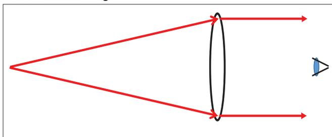
Fig. 3. Rays diverging from the focal distance (in front of the lens) passing through a convex lens emerge as parallel rays. The result is that the observer cannot see any image at all.
