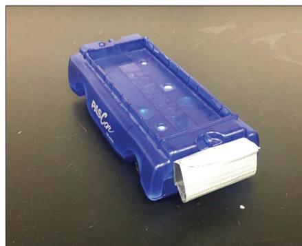
Fig. 4. Duct tape rolled into a cylinder, sticky-side out, attached to the magnetized end of a cart.
