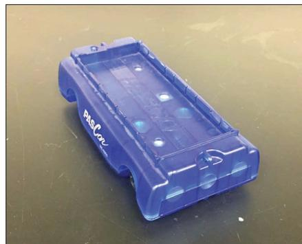
Fig. 3. The circles (disks) embedded in the end of the cart are magnets.
