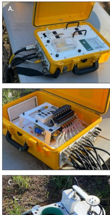
Figure 1. SR measurement equipment. A. LI-8100, IRGA, B. LI-8150, multiplexer, C. LI-8150-104, long-term chamber
