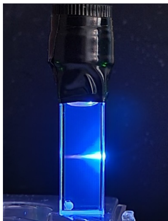
Illustration 1. Image of upconverting solution containing PdOEP, Pyrenebutanol, and PTEA at a wt% ratio of 1:30:1 PdOEP:Pyrenebutanol:PTEA
