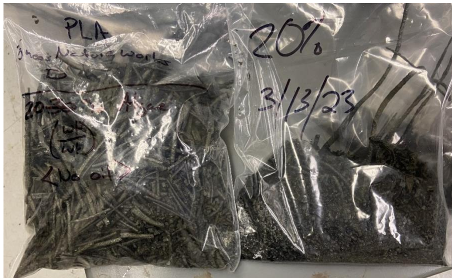
Figure 9. 20 wt.% Algae-PLA hm (left) and 20 wt.% Algae-PLA cm (right).
