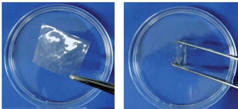
Fig. 2 Water-solubilization of the polyimide film derived from 4,4'-diamino-truxillate potassium salts. Left: transparent polyimide film, right: polyimides immersed in water.
