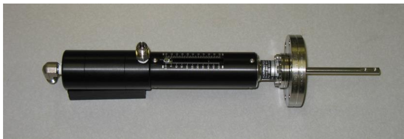
Figure 6.9 Pneumatic Linear Feedthrough before installation (above) and Linear Feedthrough after installation with pneumatic control lines and solenoid control valve (below).
