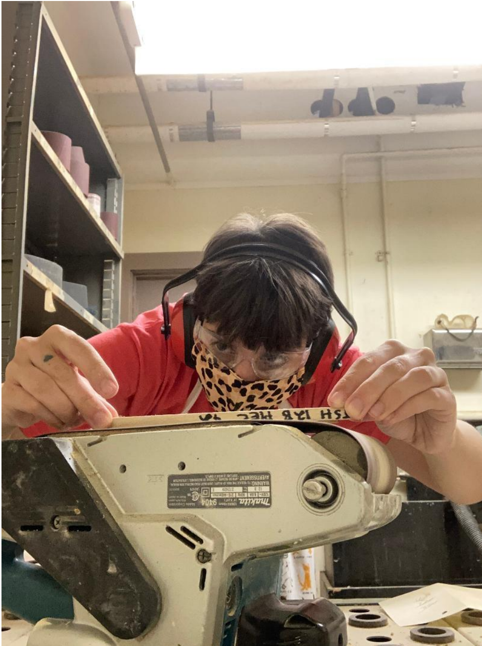
Figure 2.8 Sanding Core Samples
