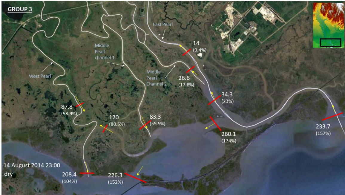
Figure 4.7 : The discharge distribution at Group 3 of the river section, showing the Middle Pearl channels, and the three outlets of Pearl: Little Lake, East, and West Pearls for the dry period in August 2014. Numbers show the flowrate in m 3 /s at identified red cross-sections and values in parenthesis show the percentage of that flow with respect to the flow in Bogalusa.
