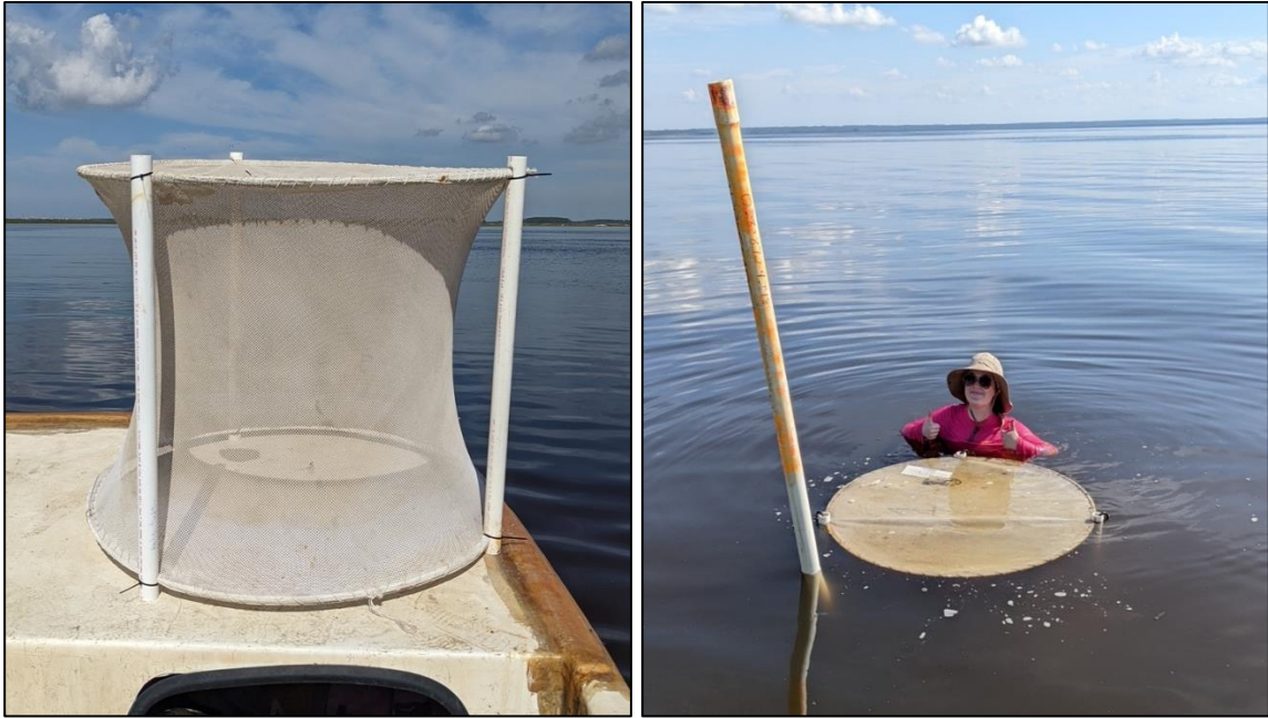
Figure 4. Mesh cages used for the brown shrimp growth experiment in the Grand Bay NERR shown out of the water (left) and in the water with a marker pole (right). Cages were 1.07-m in diameter and 0.76-m tall with 3.2-mm mesh. 15 cages were deployed with 5 in each habitat type ( Ruppia maritima , Halodule wrightii , and unvegetated bottom).
