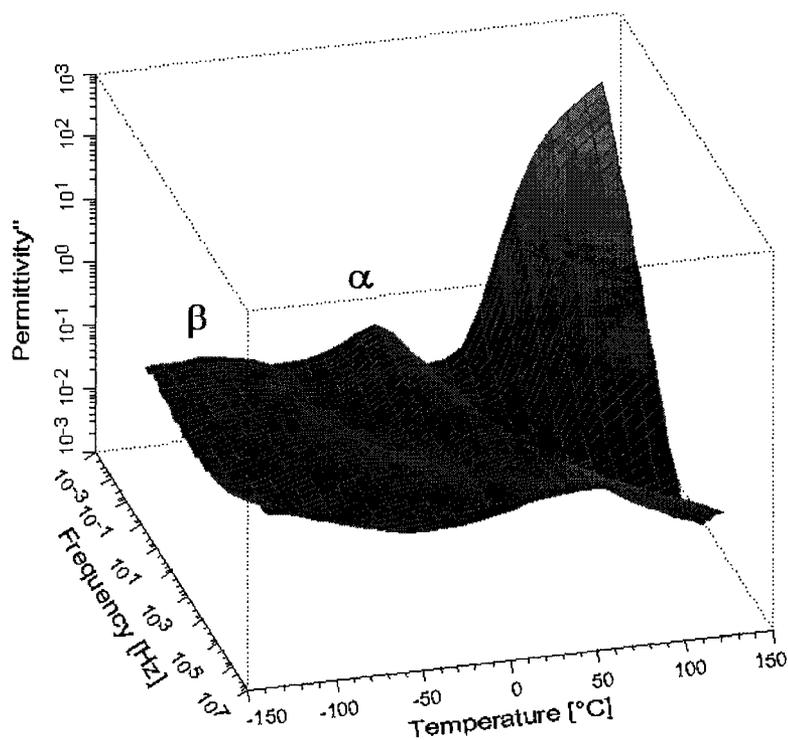
**Figure 0-4.**  $\epsilon''$ - $f$ - $T$  surface for a 1200 EW unmodified, as-received Nafion<sup>®</sup> precursor sulfonyle fluoride film.
