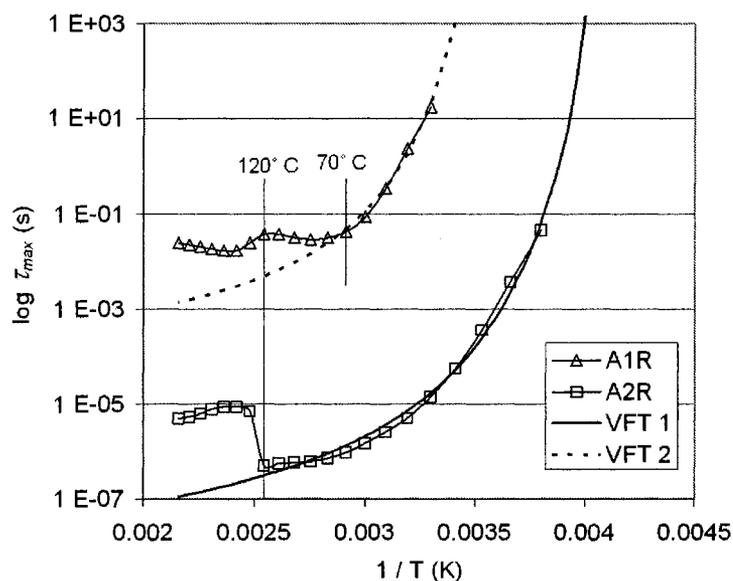
**Figure 0-7.**  $\log \tau_{\text{max}}$  vs.  $1/T$  plots for the A1R and A2R relaxations for a Nafion<sup>®</sup> sulfonyl fluoride film reacted symmetrically with 1,4 BDA to a depth of  $10\mu\text{m}$  from both surfaces without prior heat treatment. Superimposed curves are VFT equation fits to each relaxation across the appropriate lower temperature ranges.
