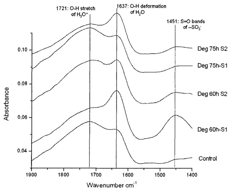
**Figure 0-15.** FTIR-ATR spectrum of as-received Nafion<sup>®</sup> and Nafion<sup>®</sup> degraded for 60 and 75h.
