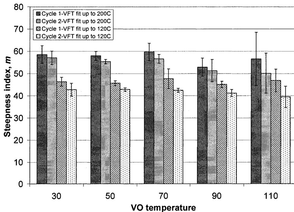
**Figure 0-18.** Fragility indices averaged at each vacuum oven temperature with one standard deviation error bars. Values from VFT equations fit with  $\tau_0 = 2 \times 10^{-7}$  s or VFT equations fit up to 200° C and  $\tau_0 = 3 \times 10^{-8}$  s for VFT equations fit up to 120° C.
