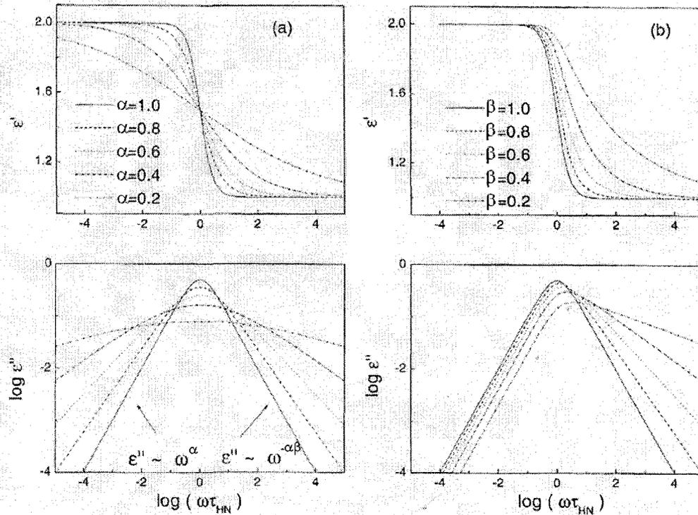
**Figure 0-14.** Complex permittivity vs.  $\log \omega\tau_{HN}$  illustrating the affect that the breadth and symmetry terms have on the relaxation (adapted from ref.<sup>24</sup>).
