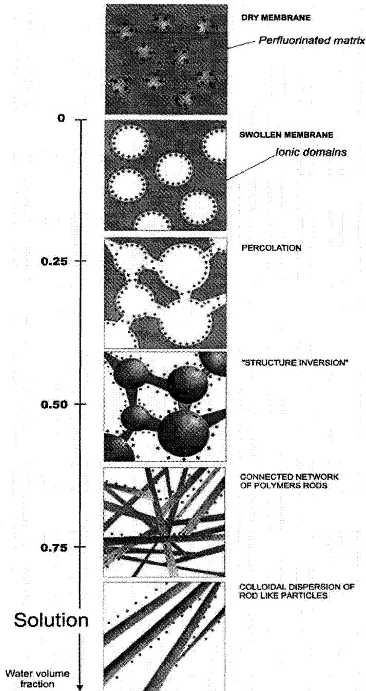
**Figure 0-4.** Gebel's schematic of morphological rearrangement due to the hydration Nafion<sup>®</sup> going from the dry to the dissolved state (adapted from ref.8).
