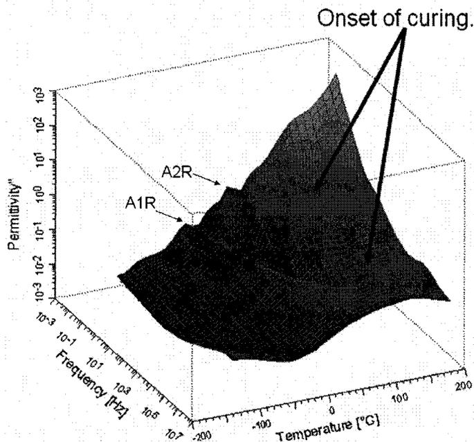
**Figure 0-6.**  $\epsilon'' - f - T$  surface for a Nafion<sup>®</sup> precursor sulfonyl fluoride film reacted symmetrically with 1,4 BDA to a depth of  $10\mu\text{m}$  from both surfaces without prior heat treatment. 'Onset of curing' refers to the effect of heating in the BDS sample cell.
