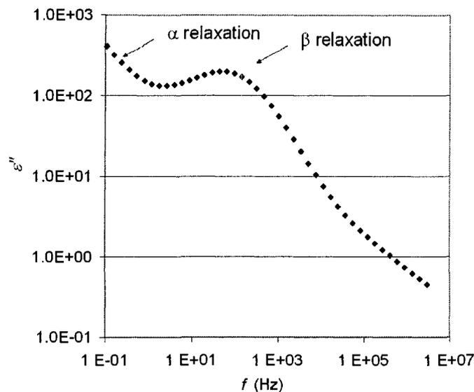
**Figure 0-2.** A typically relaxation plot of  $\log_{10}\epsilon''$  vs.  $\log f$  for H<sup>+</sup> Nafion that was chemically degraded for 75h.
