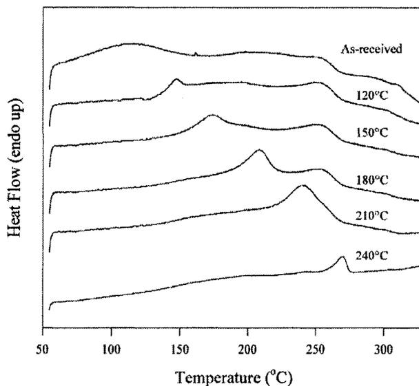
**Figure 0-7.** DSC thermogram of Cs<sup>+</sup> form 1100EW Nafion<sup>®</sup> annealed for 2h at the temperatures indicated above each trace (adapted from ref.<sup>15</sup>).
