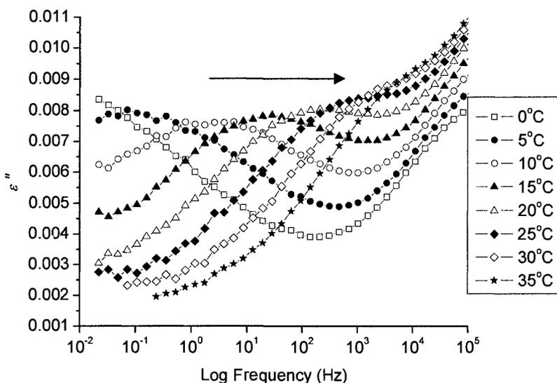
**Figure 0-10.**  $\log_{10} \epsilon''$  vs.  $\log_{10} f$  for 1200 EW films illustrating  $\alpha$  relaxation peaks at indicated temperatures with dc conductivity subtracted. Arrow indicates direction of peak shift with increasing temperature.
