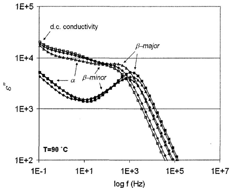
**Figure 0-19.** BDS spectra of  $\log \epsilon''$  vs.  $\log f$  at  $90\text{ }^{\circ}\text{C}$  for  $\text{H}^+$  Nafion boiled in a) HCl (solid symbols) b)  $\text{HNO}_3$  (open symbols).
