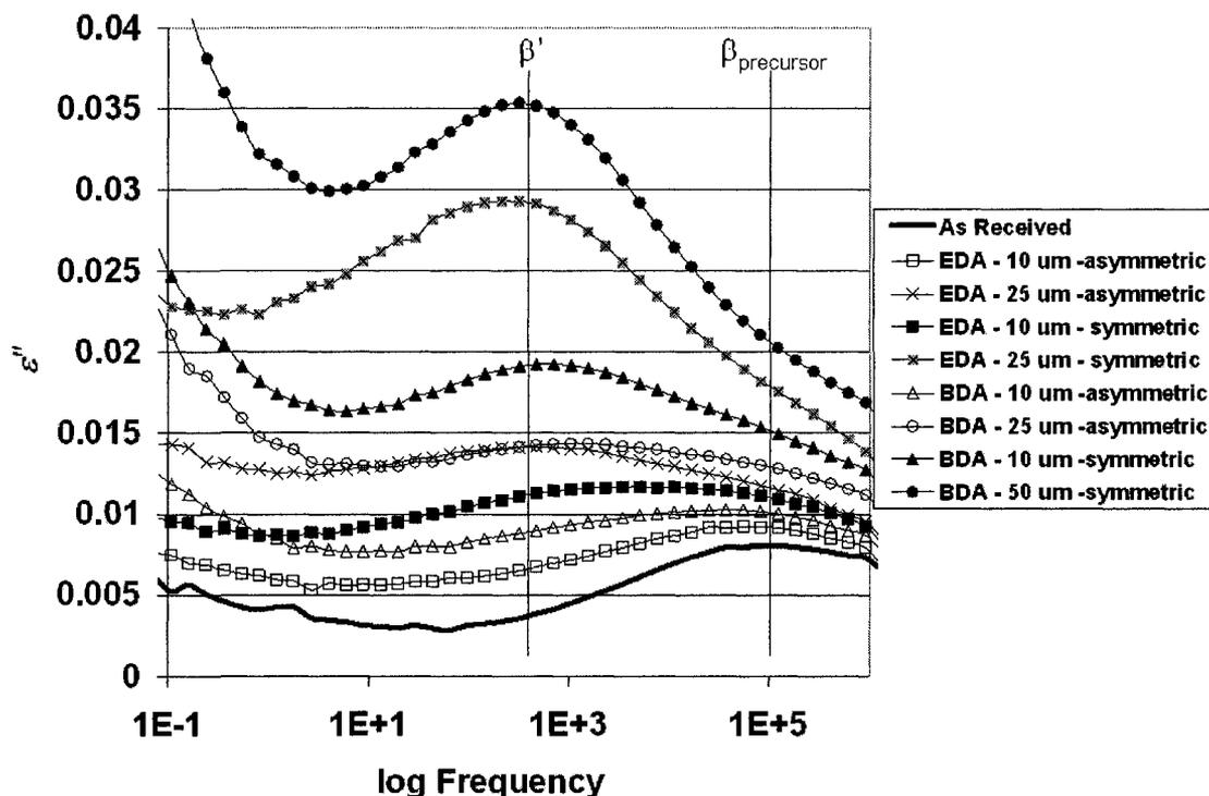
**Figure 0-14.**  $\epsilon''$  vs.  $\log f$  at  $-10\text{ }^{\circ}\text{C}$  for EDA and 1,4 BDA modified films at indicated reaction depths. The chemically unmodified sample curve (solid black) has two peaks at approximately  $10^5$  Hz. Amine modified films have an additional  $\beta'$  relaxation appearing as a shoulder at short reaction depths that sharpens with increasing reaction depth.
