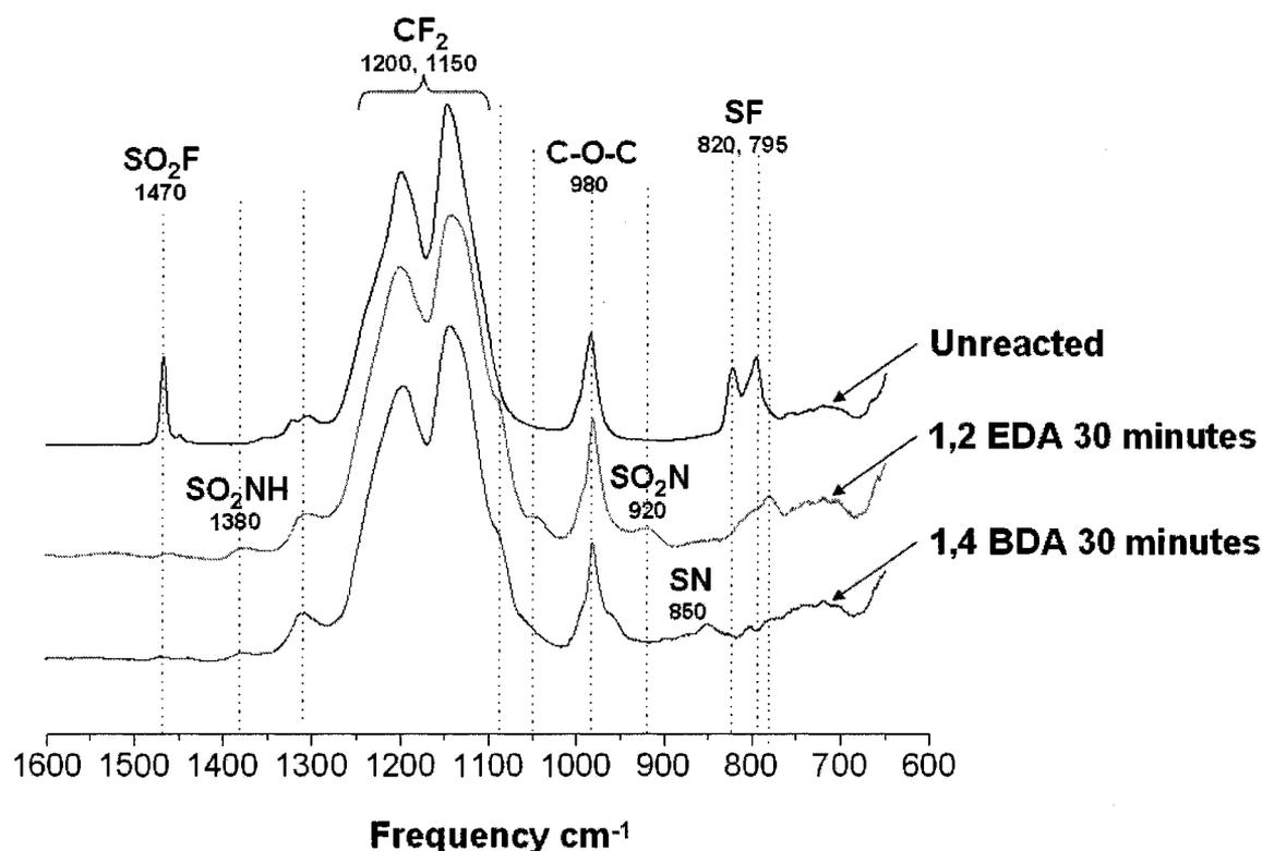
**Figure 0-2.** FTIR/ATR spectra for an unmodified Nafion<sup>®</sup> sulfonyl fluoride film and 1,2 films symmetrically reacted with EDA and 1,4 BDA for 30 min, but with no curing. Both film sides have the same spectra in each case
