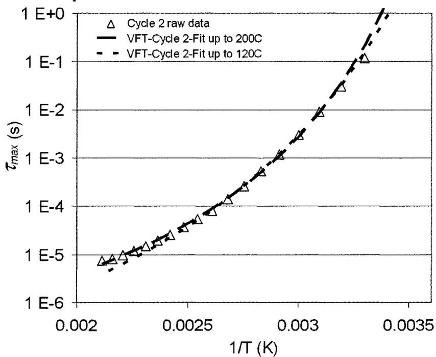
**Figure 0-16.** VFT plot of  $\log_{10} \tau_{max}$  for the  $\beta$  relaxation vs.  $1/T$  for the 2<sup>nd</sup> cycle of a VO30-IS90 sample.
