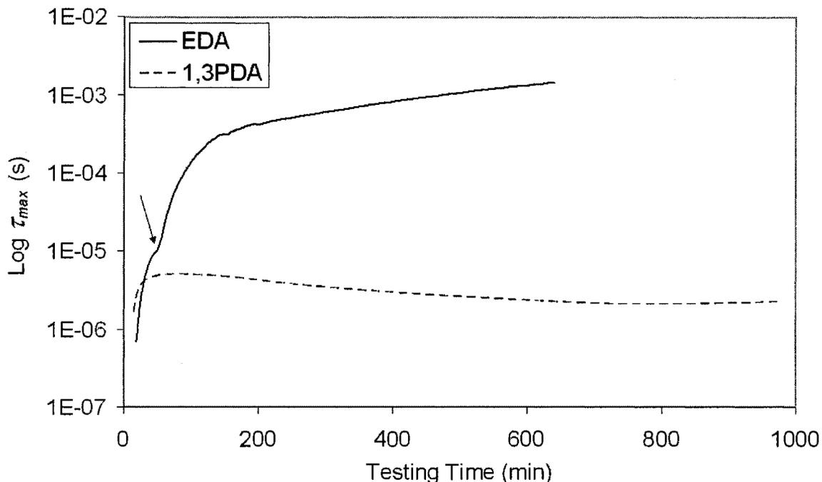
**Figure 0-10.** Log<sub>10</sub> τ<sub>max</sub> vs. BDS test time for the A1R relaxation for consecutive frequency sweep spectrum iterations at a constant temperature of 200° C for diamine modified films that were not heat cured before testing. Inflection point for the EDA curve is marked with arrow.
