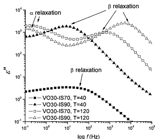
**Figure 0-6.**  $\log_{10} \epsilon''$  vs.  $\log_{10} f$  with dc contribution subtracted for 1<sup>st</sup> temperature cycle for samples VO30-IS70 and VO30-IS90 both at 40° C and 120° C.
