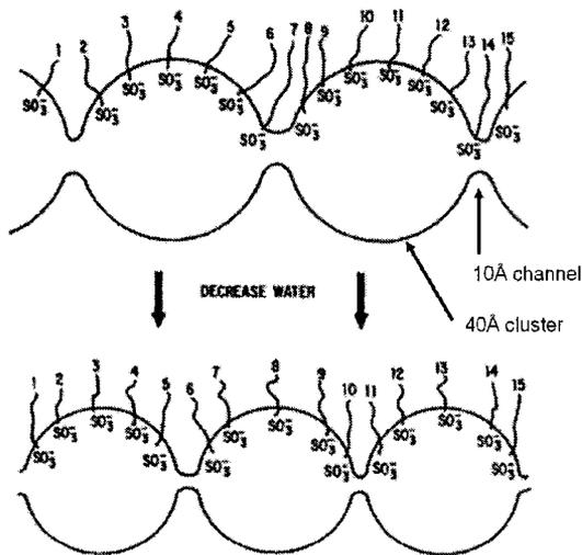
**Figure 0-2.** Redistribution of ion exchange sites into a different number of clusters in the cluster-network model upon dehydration (adapted from ref.<sup>4</sup>).
