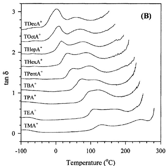
**Figure 0-8.** DMA plot of  $\tan \delta$  vs. temperature for various tetraalkylammonium counterion forms of Nafion<sup>®</sup> (adapted from ref.<sup>15</sup>).
