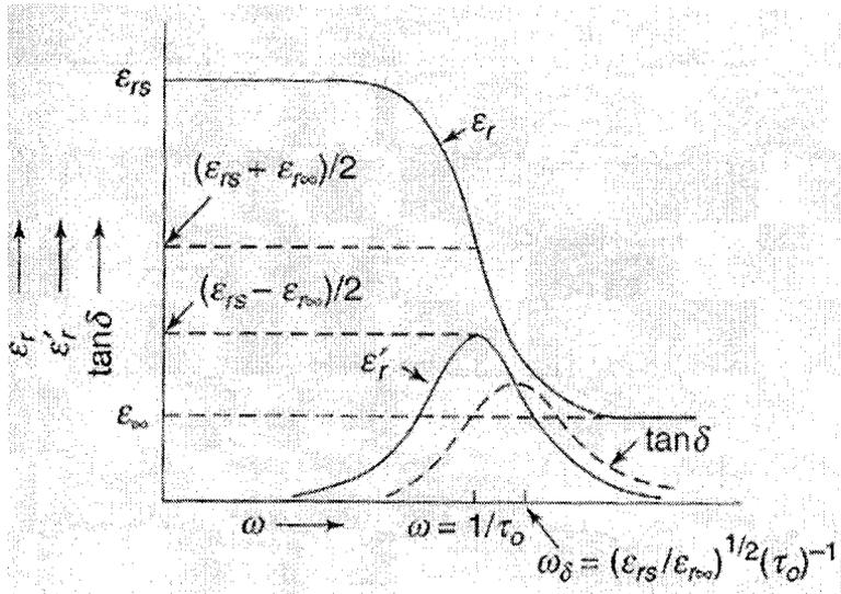
**Figure 0-13.** Typical relaxation response as a function of angular frequency (adapted from ref.<sup>22</sup>).
