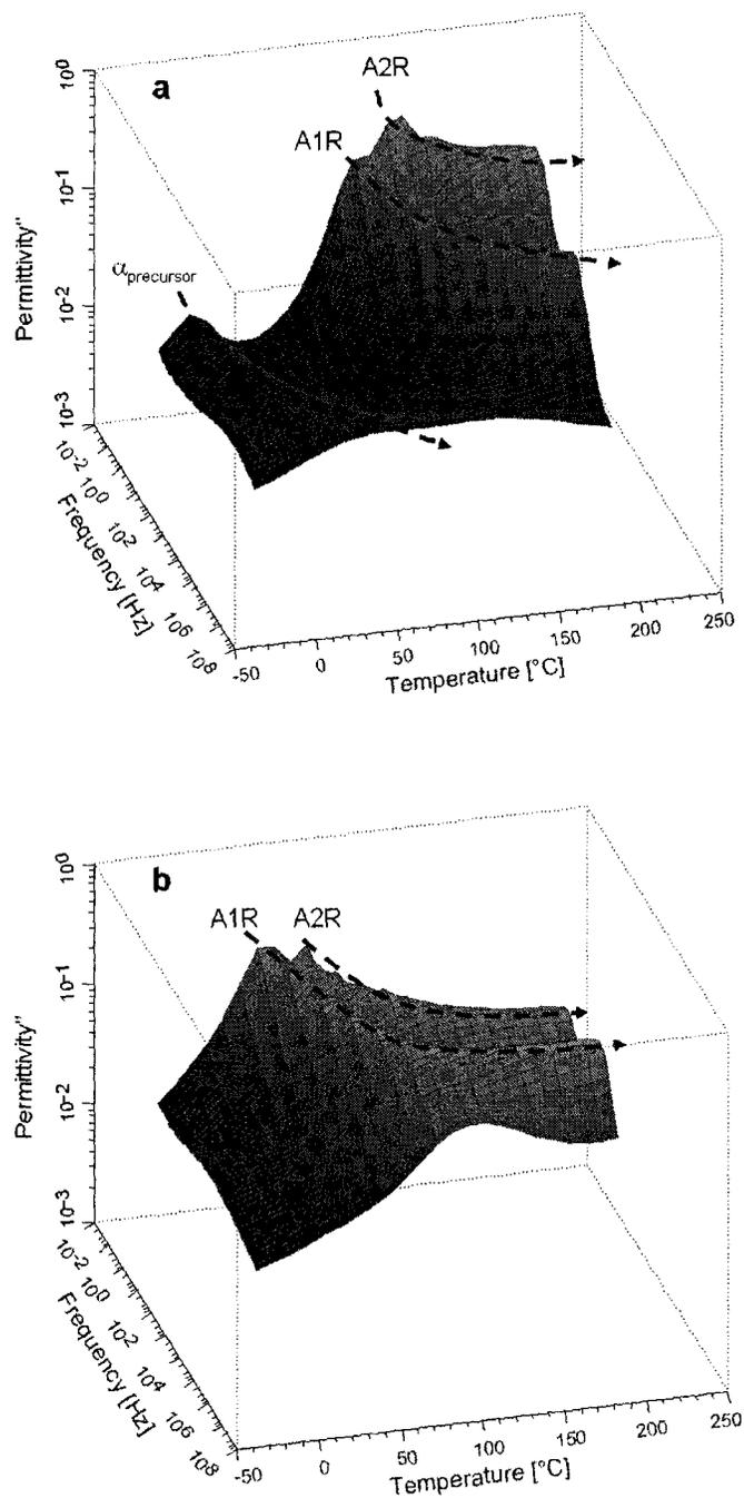
**Figure 0-8.**  $\epsilon''-f-T$  surfaces with d.c. subtracted for films cured for 1h at 200 $^{\circ}$  C before dielectric measurements: a) EDA symmetrically reacted to a depth of 10 $\mu$ m; b) 1,4 BDA symmetrically reacted to a depth of 10  $\mu$ m. The dashed black curves are the crests of the relaxation peaks at  $f_{\text{max}}$  over the range of T.
