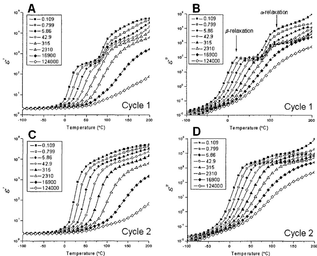
**Figure 0-5.**  $\log_{10} \varepsilon'$  vs.  $T$  (left) and  $\log_{10} \varepsilon''$  vs.  $T$  of VO30-IS70 at indicated frequencies (Hz). A series of frequency sweeps were performed at  $10^\circ \text{C}$  increments from  $-130$  to  $200^\circ \text{C}$  after *in situ* drying. Plots A,B are for cycle 1 and plots C,D are for cycle 2.
