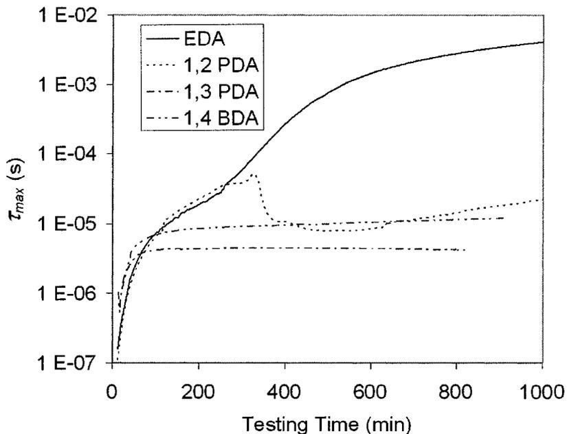
**Figure 0-11.**  $\text{Log}_{10} \tau_{\text{max}}$  vs. test time in the BDS instrument for the A1R relaxation for consecutive frequency sweep iterations performed at the constant temperature  $170^\circ \text{C}$  for amine modified films that were not heated (cured) before testing.
