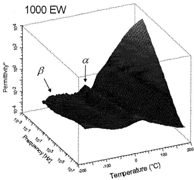
**Figure 0-1**  $\epsilon''$  -  $f$  -  $T$  response surface for a 1000 EW Nafion<sup>®</sup> sulfonfyl fluoride precursor film.
