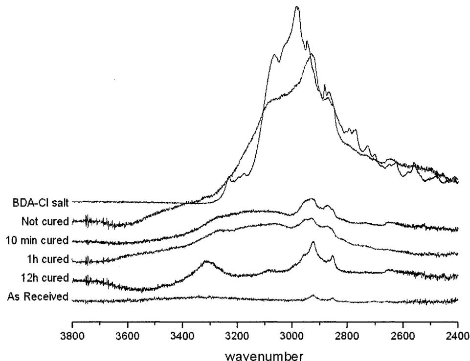
**Figure 0-3.** FTIR/ATR spectra in the region 3600-2600  $\text{cm}^{-1}$  for unmodified Nafion<sup>®</sup> sulfonyl fluoride, a small molecule model salt (1,4 diaminobutane-dihydrochloride) and films symmetrically reacted with 1,4 BDA and cured for 0, 10, 60 and 720 min.
