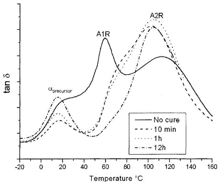
**Figure 0-17.** DMA  $\tan \delta$  vs. temperature at 1 Hz for indicated cure times for 1,4 BDA films symmetrically reacted to a depth of  $10\mu\text{m}$ .
