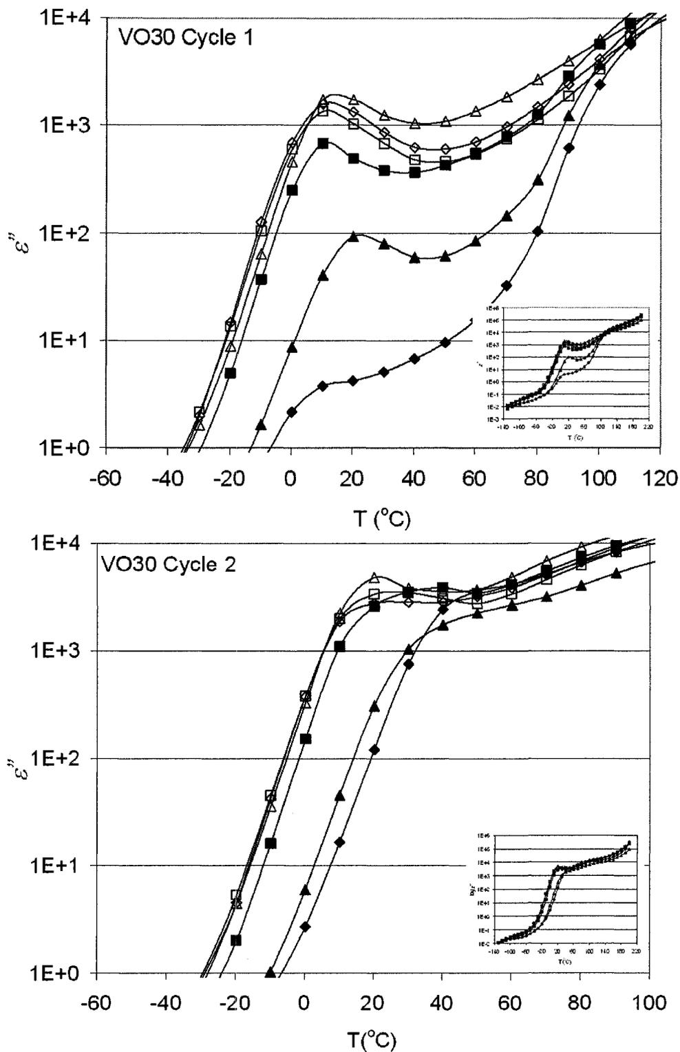
**Figure 0-10.**  $\text{Log}_{10} \varepsilon''$  vs.  $T$  ( $^{\circ}\text{C}$ ) for samples dried in vacuum at  $30^{\circ}\text{C}$ , then tested *in situ* in the BDS at  $70^{\circ}\text{C}$  (filled triangles) and  $90^{\circ}\text{C}$  (open squares). Left plot designates first temperature cycle and right plot designates the second temperature cycle. Different shapes designate different specimens.
