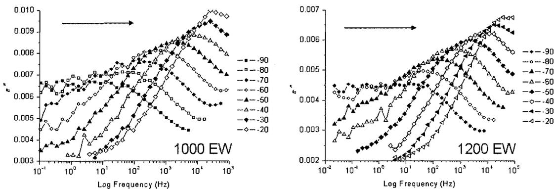
**Figure 0-12.** 2-D  $\epsilon''$  vs.  $f$  plots illustrating the  $\beta$  relaxation for 1000 and 1200EW samples from  $-90$  to  $-20^\circ\text{C}$ . dc conductivity is not present at these temperatures. Arrow indicates the peak shift direction with increasing temperature.
