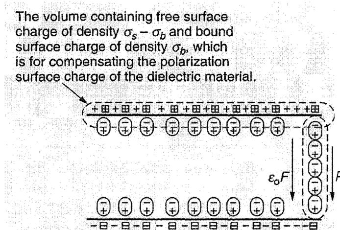
**Figure 0-10.** Dielectric material sandwiched between equal and opposite charged parallel plates. The + and - symbols represent free positive and negative whereas the boxed charges represent bound charges distributed on the metal electrodes. The free charges produce the electric flux density  $\epsilon_0 F$  whereas the bound charges produce the polarization  $P$  within the dielectric material (adapted from ref.<sup>22</sup>).
