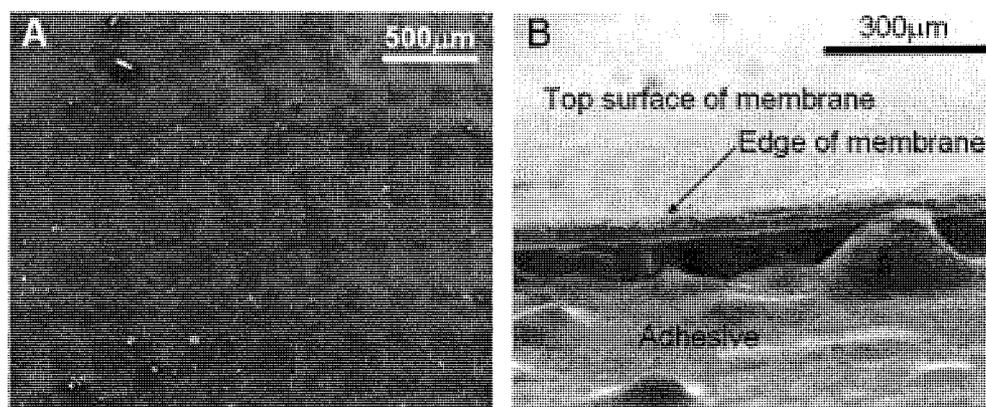
**Figure 0-4.** SEM scans of 45h film exposure to Fenton's reagent solution A) top, B) side views. Adhesive was used to attach the Nafion H<sup>+</sup> membrane to the SEM stage.
