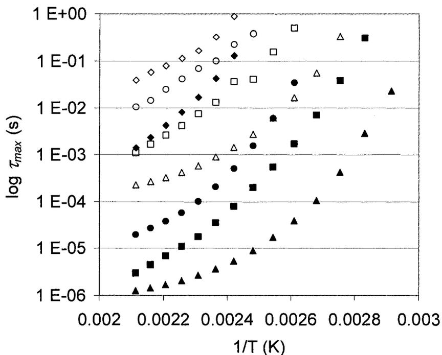
**Figure 0-13.**  $\log \tau_{max}$  vs.  $1/T$  for films symmetrically reacted to  $10\mu\text{m}$  depth and cured for 12h : EDA ( $\diamond$ ), 1,2 PDA ( $\circ$ ), 1,3 PDA ( $\Delta$ ), 1,4 BDA ( $\square$ ). Closed symbols are A1R and open symbols are A2R.
