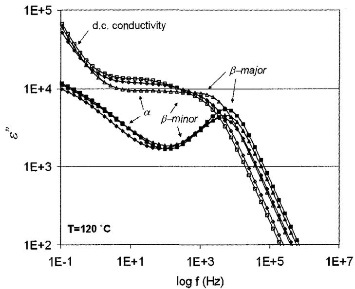
**Figure 0-20.** BDS spectra of  $\log \epsilon''$  vs.  $\log f$  at  $120\text{ }^{\circ}\text{C}$  for  $\text{H}^+$  Nafion boiled in a) HCl (solid symbols) b)  $\text{HNO}_3$  (open symbols).
