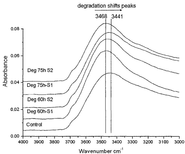
**Figure 0-14.** FTIR-ATR spectrum O-H stretch for as-received Nafion<sup>®</sup> and Nafion<sup>®</sup> degraded for 60 and 75h.
