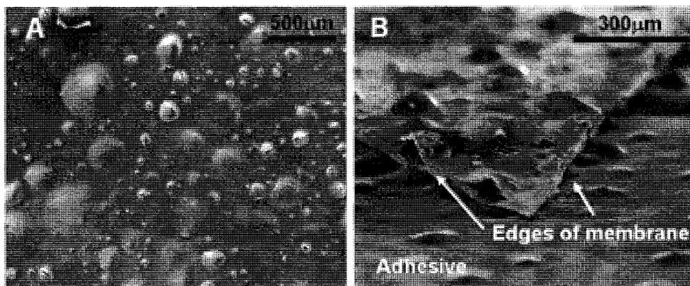
**Figure 0-5.** SEM scans of 60h film exposure to Fenton's reagent solution A) top, B) side views of two edges cut through the degraded membrane. Cuts made post-degradation.
