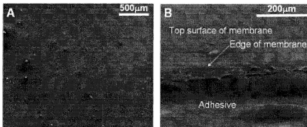
**Figure 0-3.** SEM scan of as-received film with no exposure to Fenton's reagent solution. Adhesive was used to attach the Nafion H<sup>+</sup> membrane to the SEM stage.
