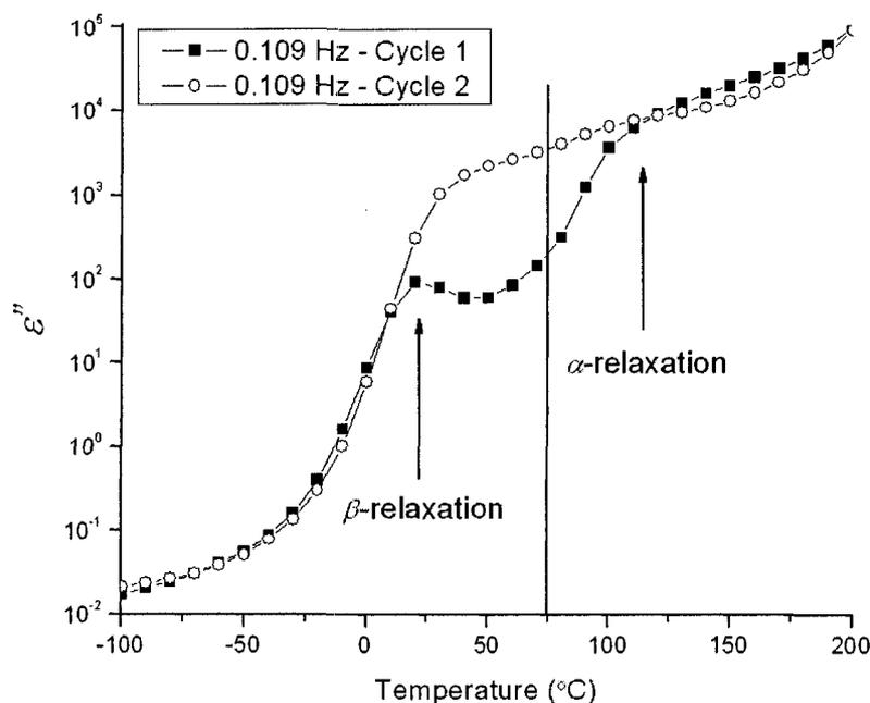
**Figure 0-9.**  $\text{Log}_{10} \varepsilon''$  vs.  $T$  at 0.11 Hz for two consecutive temperature cycles from  $-130$  to  $200^\circ \text{C}$  with frequency sweeps at  $10^\circ \text{C}$  increments. The temperature is held constant at each frequency sweep. Before testing, the sample was dried in a vacuum oven at  $30^\circ \text{C}$  for 12 h. Before the temperature was reduced to  $-130^\circ \text{C}$  the sample was dried at  $70^\circ \text{C}$  for approximately 9.75 h.
