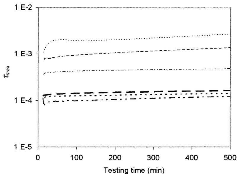
**Figure 0-4.**  $\text{Log}_{10} \tau_{max}$  for  $\beta$  relaxation vs. drying time for six VO30 samples: three dried *in situ* at 70° C (light curves, top) and three dried *in situ* at 90° C (bold curves, bottom).
