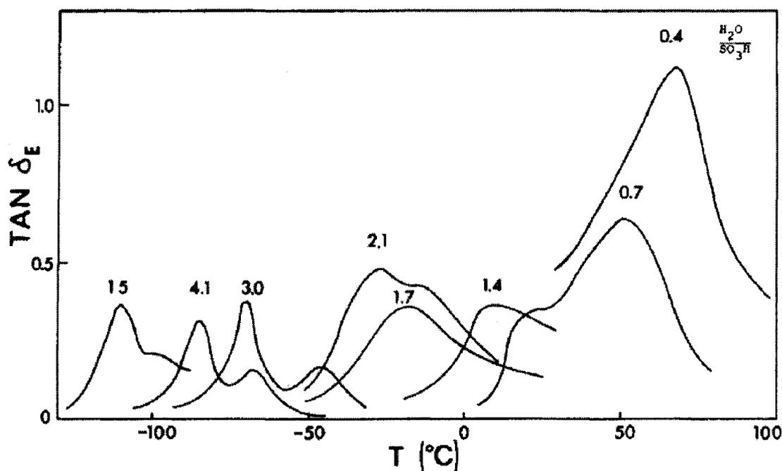
**Figure 0-6.** Dielectric loss tangent vs. temperature at various water contents at 100Hz for H<sup>+</sup>Nafion<sup>®</sup> (adapted from ref.<sup>15</sup>). The numbers corresponding to each peak represents the average number of water molecules per sulfonate group.
