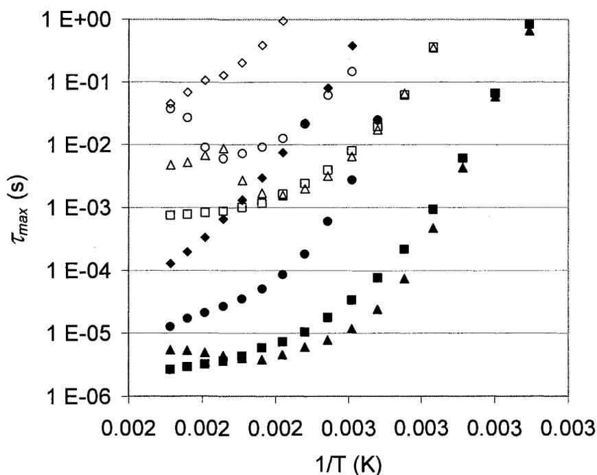
**Figure 0-12.**  $\log_{10}\tau_{\max}$  vs.  $1/T$  for films symmetrically reacted to  $10\mu\text{m}$  depth and cured for 1h: EDA ( $\diamond$ ), 1,2 PDA ( $\circ$ ), 1,3 PDA ( $\Delta$ ), 1,4 BDA ( $\square$ ). Closed symbols are A1R and open symbols are A2R.
