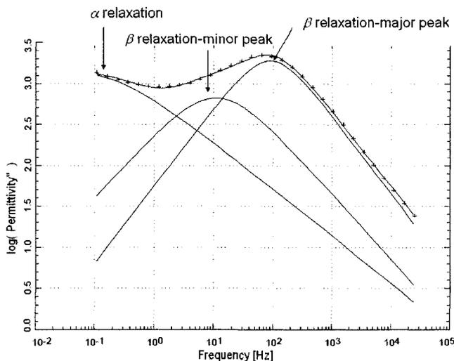
**Figure 0-8.**  $\text{Log}_{10} \epsilon''$  vs.  $\text{log}_{10} f$  for a VO30-IS90 sample at  $60^\circ \text{C}$ . The glass transition is best fit with two HN parameters. The (+) symbols are actual data points.
