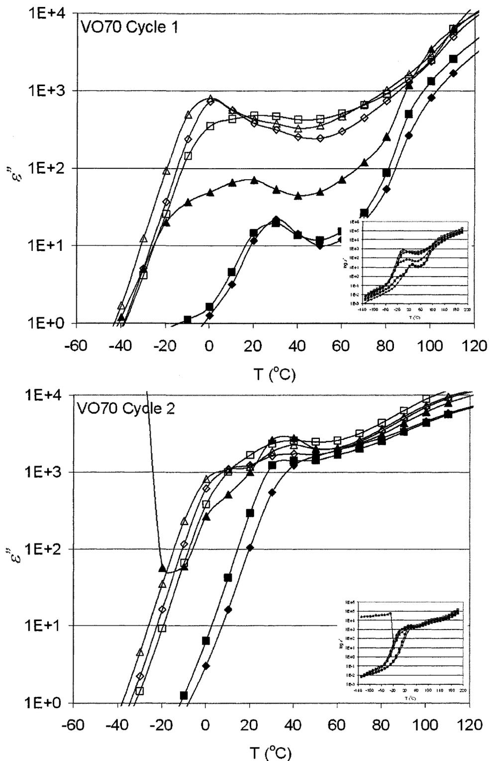
**Figure 0-12.**  $\text{Log}_{10} \varepsilon''$  vs.  $T$  ( $^{\circ}\text{C}$ ) for samples dried in vacuum oven at  $70^{\circ}\text{C}$ , then *in situ* in the BDS at  $70^{\circ}\text{C}$  (filled triangles) and  $90^{\circ}\text{C}$  (open squares). Left plot is for first temperature cycle; right plot is for second temperature cycle. Different shapes designate different samples.
