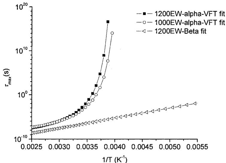
**Figure 0-15.** Fitted curves for the  $\alpha$  and the  $\beta$  relaxations illustrating the  $\alpha$ - $\beta$  merging process.
