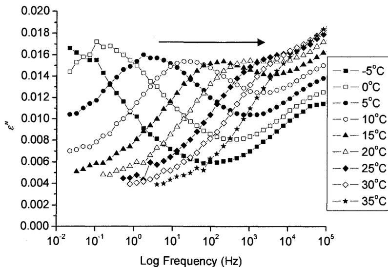
**Figure 0-9.**  $\log_{10} \epsilon''$  vs.  $\log_{10} f$  for 1000EW films illustrating  $\alpha$  relaxation peaks at indicated temperatures with dc conductivity subtracted. Arrow indicates direction of peak shift with increasing temperature.
