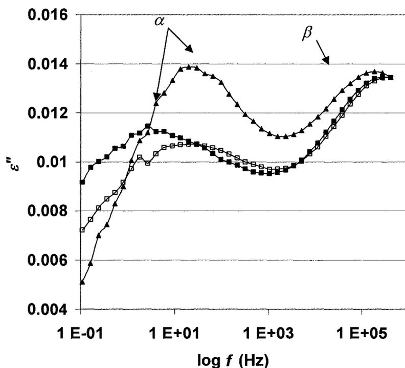
**Figure 0-11.**  $\epsilon''$  vs.  $\log f$  for 1200EW (squares) and 1000EW (triangles) films. Solid shapes are for frequency sweeps at  $10^\circ$  C and open shapes are for a sweep at  $13^\circ$  C.
