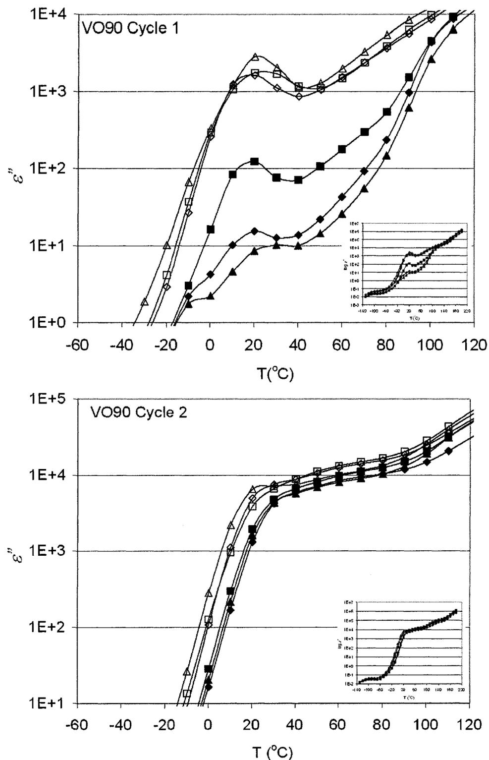
**Figure 0-13.**  $\text{Log}_{10} \epsilon''$  vs.  $T$  ( $^{\circ}\text{C}$ ) for samples dried in vacuum oven at  $90^{\circ}\text{C}$ , then *in situ* in BDS at  $70^{\circ}\text{C}$  (filled triangles) and  $90^{\circ}\text{C}$  (open squares). Left plot is for first temperature cycle; right plot is for second temperature cycle. Different shapes designate different specimens.
