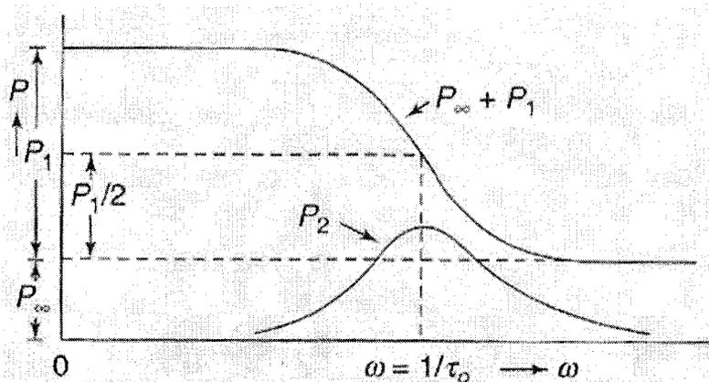
**Figure 0-12.** Storage and loss polarization responses vs. angular frequency  $= \omega = 2\pi F$  where the complex variable  $P^*(\omega) = P_\infty + P_1 + P_2$ .  $P_\infty + P_1$  contains the storage component  $P_1$  and the loss component is  $P_2$  (adapted from ref.<sup>22</sup>).
