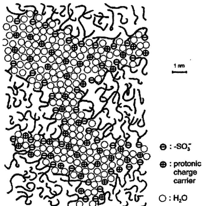
**Figure 0-5.** Kreuer’s illustration of Nafion<sup>®</sup>’s morphology which has three phases, consisting of ionic and non-ionic phases with a “fuzzy” interface and crystallinity in the non-ionic phase.
