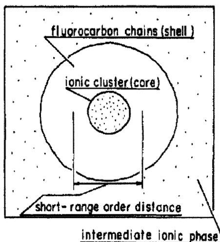
**Figure 0-3.** A schematic of the core-shell model as originally illustrated by Fujimura (adapted from ref.<sup>6</sup>).
