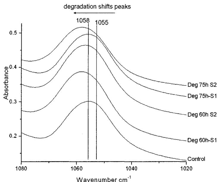
**Figure 0-12.** ATR-IR spectrum of the SO<sub>3</sub><sup>-</sup> symmetric stretch as received Nafion<sup>®</sup> and Nafion<sup>®</sup> degraded for 60h and 75h highlighting the shift to higher wavenumber with degradation.
