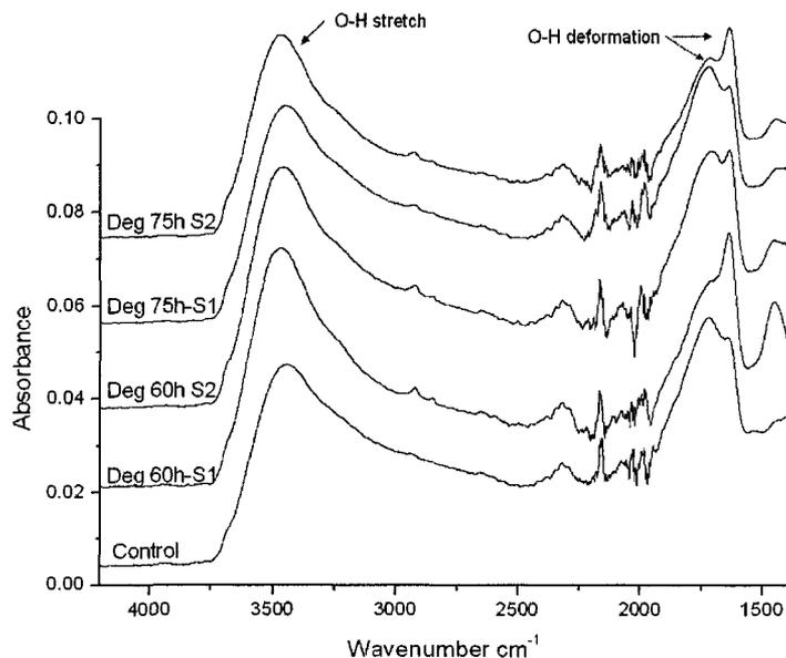
**Figure 0-13.** FTIR-ATR spectrum highlighting the O-H absorption of as received Nafion<sup>®</sup> and Nafion<sup>®</sup> degraded for 60 and 75h.
