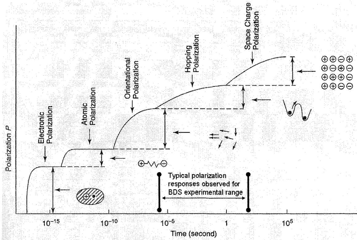
**Figure 0-11.** Spectrum of polarization mechanism time scales. The typical BDS frequency test window corresponds, approximately, to  $10^{-6}$  to  $10^2$  sec (adapted from ref.<sup>22</sup>).
