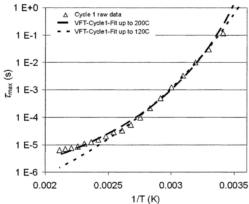
**Figure 0-15.** VFT plot of  $\log_{10} \tau_{max}$  for the  $\beta$  relaxation vs.  $1/T$  for the 1<sup>st</sup> cycle of a VO30-IS90 specimen.
