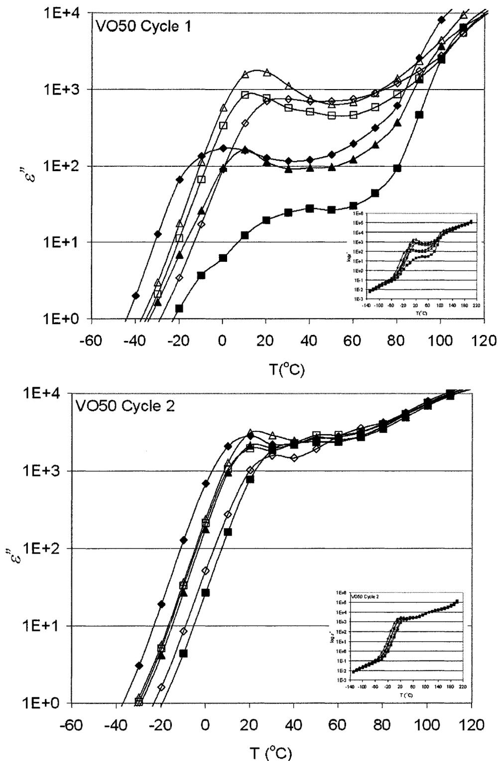
**Figure 0-11.**  $\log_{10} \epsilon''$  vs.  $T$  (°C) for samples dried in the vacuum oven at 50 °C and then *in situ* in the BDS at 70 °C (filled triangles) and 90 °C (open squares). The left plot is for the first temperature cycle and the right plot is for the second cycle. Different shapes designate different specimens.
