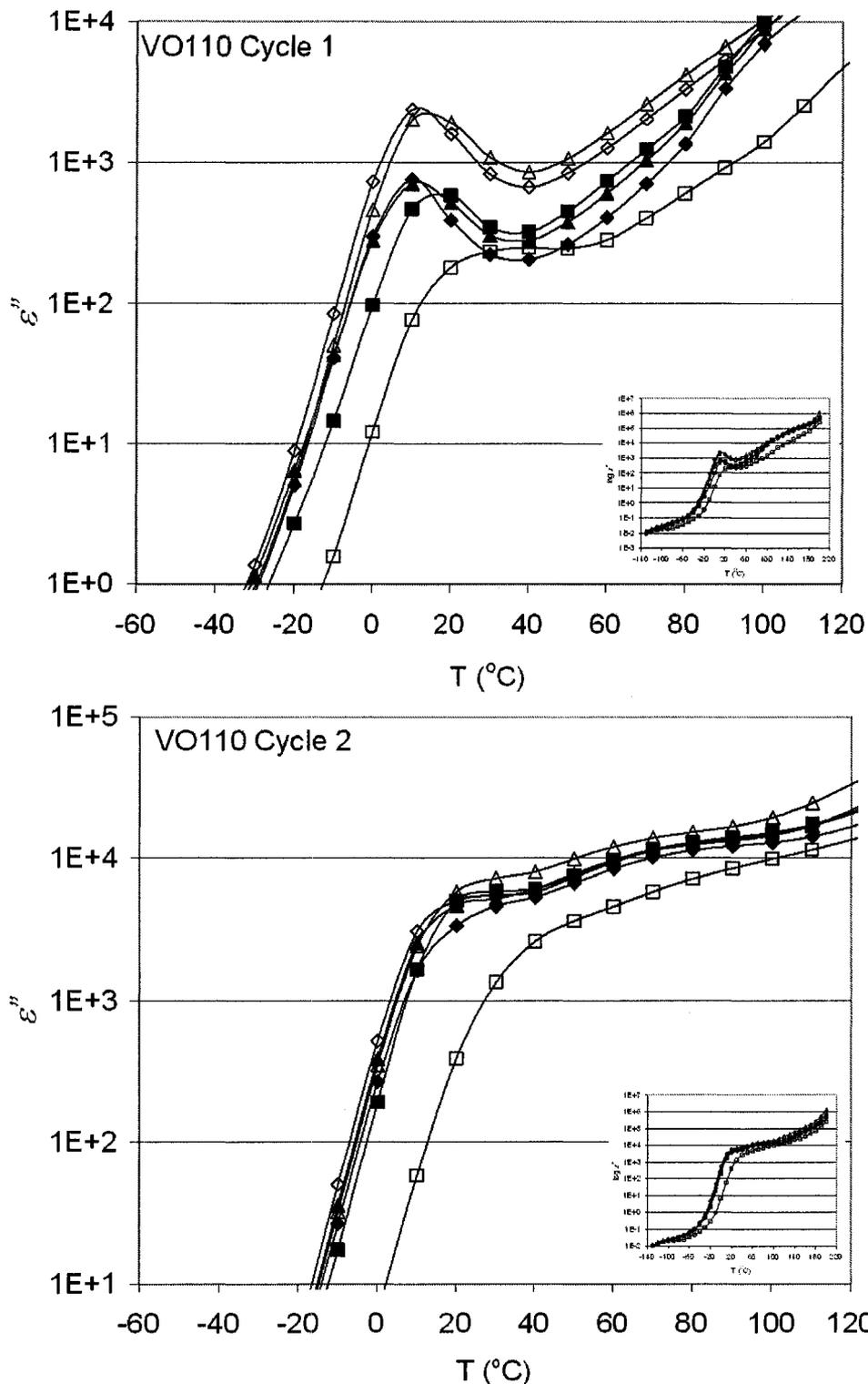
**Figure 0-14.**  $\log_{10} \varepsilon''$  vs.  $T$  ( $^{\circ}\text{C}$ ) for samples dried in vacuum oven at  $110^{\circ}\text{C}$ , then *in situ* in BDS at  $70^{\circ}\text{C}$  (filled triangles) and  $90^{\circ}\text{C}$  (open squares). Left plot is for 1<sup>st</sup> temperature cycle; right plot is for 2<sup>nd</sup> temperature cycle. Different shapes designate different specimens.
