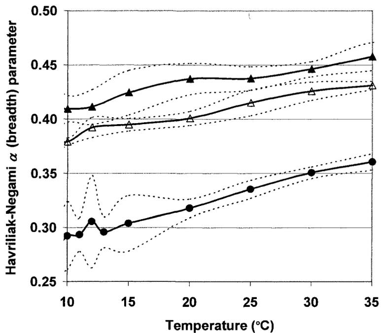
**Figure 0-8.** Average  $\alpha$  values for the  $\alpha$  relaxation obtained from H-N equation fits to  $\epsilon''$  vs.  $f$  data at each respective temperature. Triangles represent 1000 EW represented as solid points and 1000 EW CS represented as open points. The 1200 EW is designated by the solid circles. The dashes indicate one standard deviation from the average.
