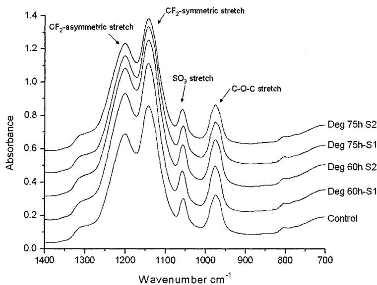
**Figure 0-11.** ATR-IR spectrum of as-received Nafion<sup>®</sup> and Nafion<sup>®</sup> degraded for 60 and 75h.
