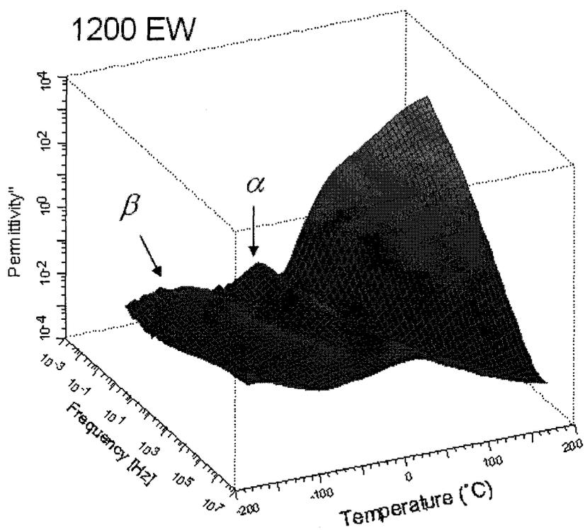
**Figure 0-2.**  $\epsilon'' - f - T$  response surface for a 1200EW Nafion<sup>®</sup> sulfonyl fluoride precursor film.
