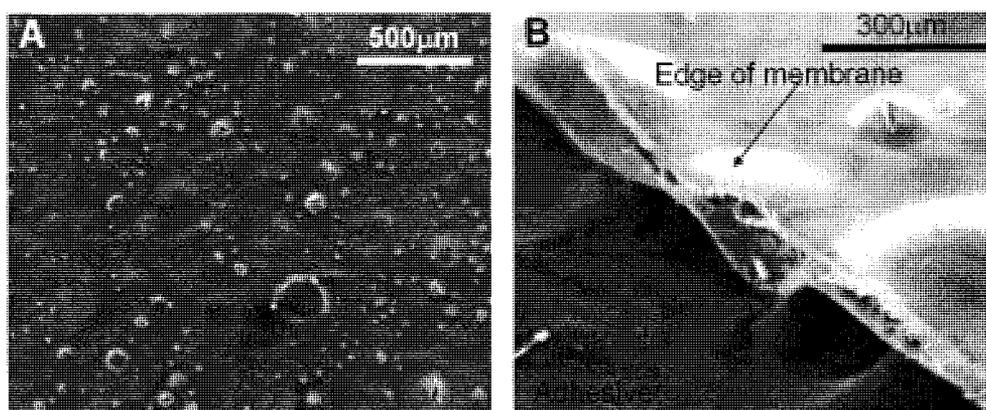
**Figure 0-6.** SEM scans of 75h film exposure to Fenton's reagent solution A) top, B) side views.
