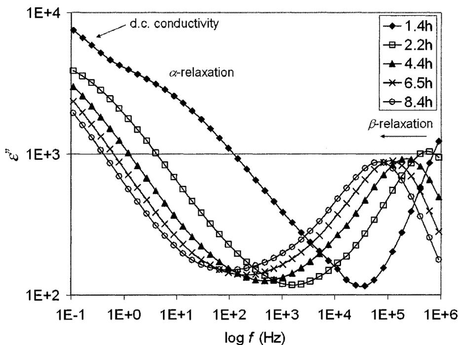
**Figure 0-2.**  $\text{Log}_{10} \varepsilon''$  vs.  $\text{log}_{10} f$  for *in situ* membrane drying at  $70^\circ\text{C}$  for different times after exposure to atmospheric moisture for  $\sim 5$  min.
