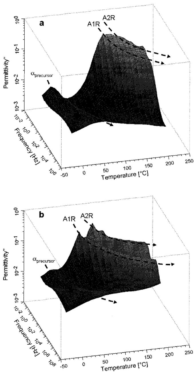
**Figure 0-9.**  $\epsilon'' - f - T$  surfaces with d.c. conductivity subtracted for films cured for 12h at 200° C before dielectric measurements: a) EDA symmetrically reacted to a depth of 10 $\mu\text{m}$ ; b) 1,4 BDA likewise symmetrically reacted to a depth of 10 $\mu\text{m}$ . The dashed black curves are the crests of the relaxation peaks at  $f_{\text{max}}$  over the range of T.
