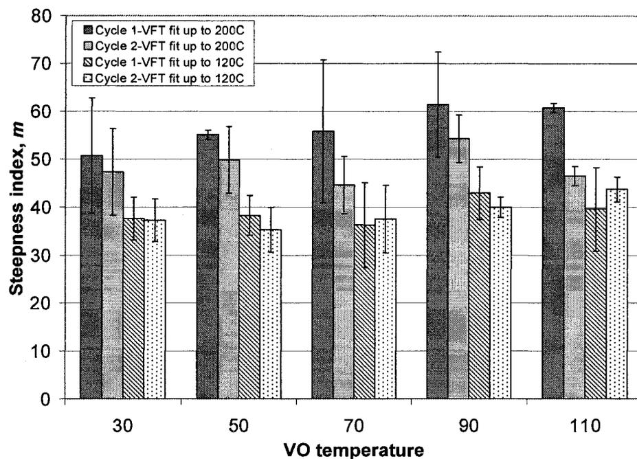
**Figure 0-17.** Fragility indices averaged at each vacuum oven (VO) temperature with error bars representing one standard deviation. These values are based on VFT equations fit with adjustable  $\tau_0$ .
