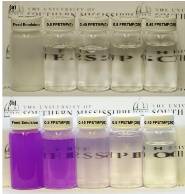
Figure A.7 Optical image of separation results (a) oil/water emulsion mixture, (b) dye contained oil/water emulsion mixture.
