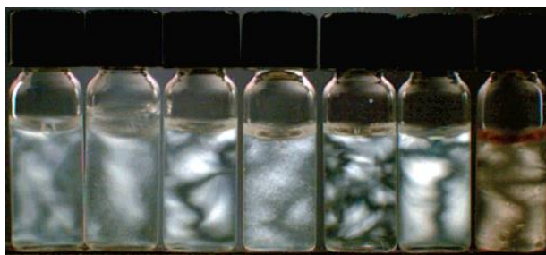
Figure 1.4 Dispersion of CNC through cross-polarizers from left to right: as prepared in water, freeze-dried and re-dispersed in water, DMF, DMSO, NMP, formic acid and m-cresol
