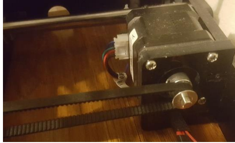
Figure 3.10 Y Axis Motor for Prusa i3 3D Printer
