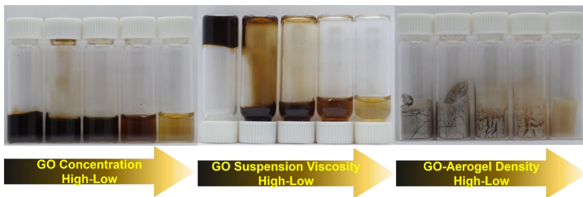
Figure B.2 Digital images of GO aqueous suspensions of varying concentrations (from left to right: 10, 5, 2.5, 1, and 0.3 mg/mL) and the resulting GO aerogels.
