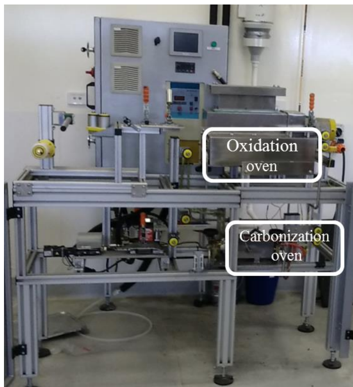
Figure 2.7 Carbon fiber simulator at Carbon Nexus with labeled oxidation and carbonization ovens.
