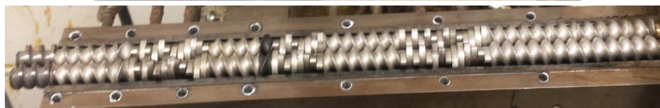
Figure 6.1 Images of (top) continuous reactor and (bottom) twin screw design used.
