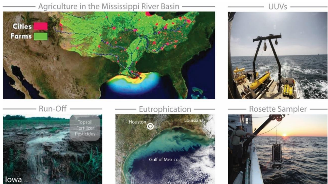
Figure 1.1 NOAA map highlighting the Gulf of Mexico run-off contributions from farms (green) and cities (red). Iowa farmland agricultural run-off. TX/LA Gulf Coast, an area of hypoxic waters (“dead zone”). Unmanned undersea vehicles (UUV). Rosette sampler: used to collect deep ocean seafloor samples and has an attached sensor package, known as a CTD (conductivity, temperature, and depth) device.
