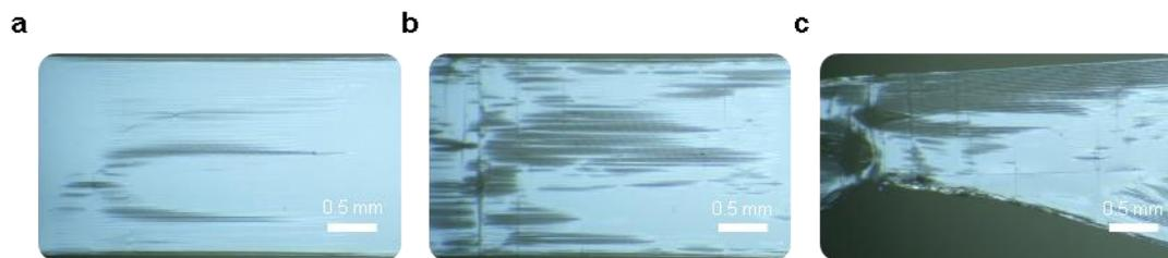
Figure B.6 Optical images of 19 nm FS PS with tensile strain of a) 1.6%, b) 2.3%, and c) 3.5%. Gage length is 8 mm.
