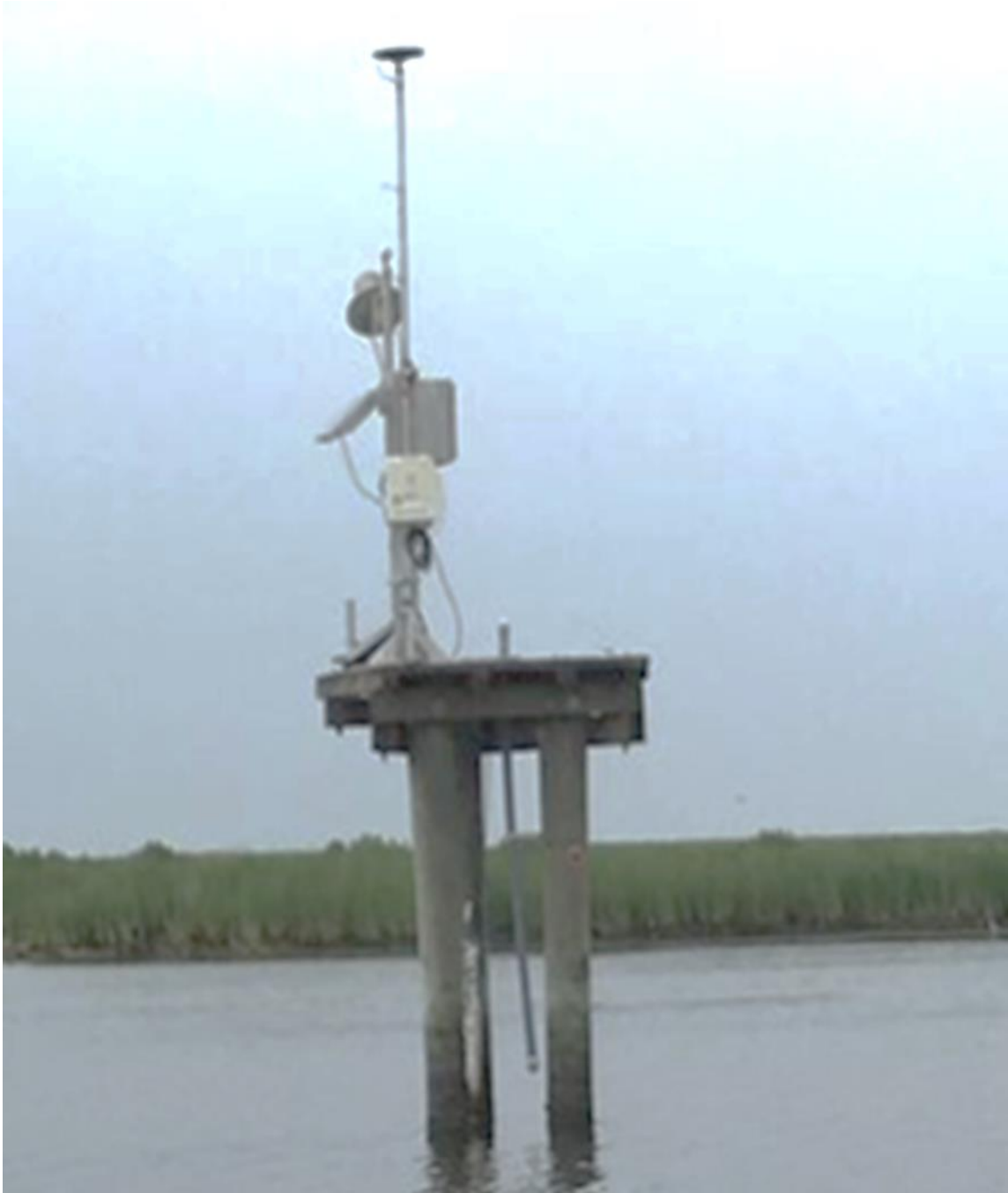
Figure 2.5 GNSS setup at Delacroix station
