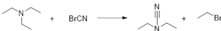
Figure 1.4 During the von Braun reaction cyanogen bromide reacts with a tertiary amine yielding an alkyl bromide and a disubstituted cyanamide.
