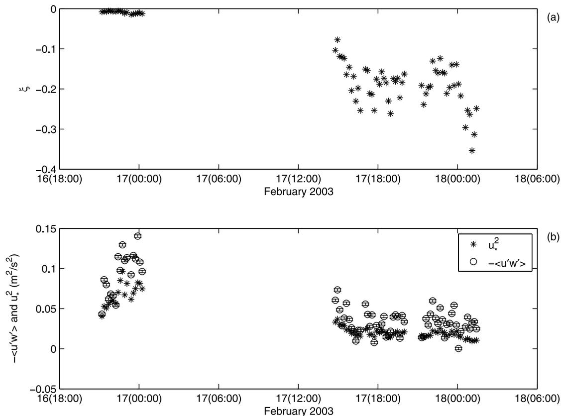
**Figure 5.** Wind stress calculation results: (a) the stability parameter  $\xi (= z/L)$ , in which  $L$  is the Monin-Obukhov length and  $z$  is the measurement height, and (b) inertial dissipation ( $u_*^2$ ) and eddy correlation ( $-\langle u'w' \rangle$ ) wind stresses with time. (In the figure,  $-\langle u'w' \rangle$  represents  $-u'w'$  in the text.) The error bars represent motion correction residual errors. Time shown in figure is UTC time.
