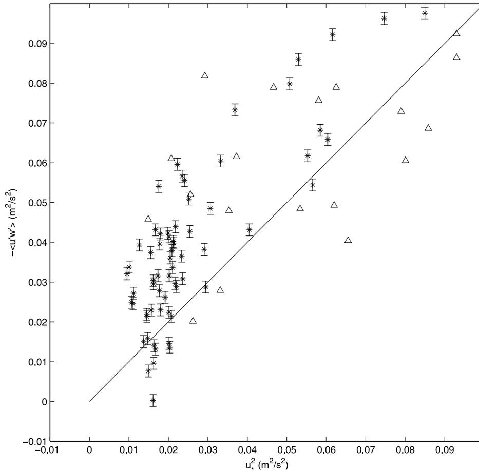
**Figure 6.** Scatterplot of  $-\langle u'w' \rangle$  and  $u_*^2$ , in which asterisks represent results of this study and triangles denote the data by *Donelan et al.* [1997] under the counter swell condition. The error bars represent motion correction residual errors.
