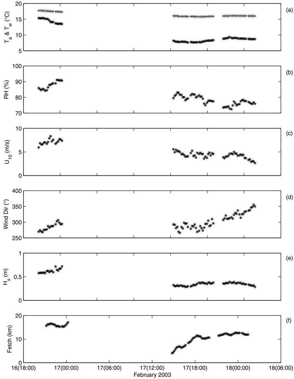
**Figure 2.** Measured atmospheric and oceanic environment parameters: (a) air (plus signs) and seawater (asterisks) temperatures, (b) relative humidity, (c) 10 m wind speed, (d) wind direction, (e) significant wave height, and (f) fetch. Time shown in figure is UTC time.
