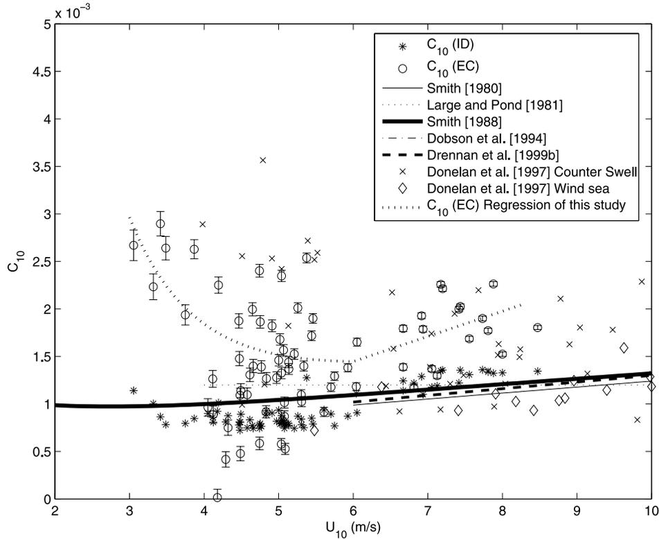
**Figure 7.** Neutral drag coefficients ( $C_{10}$ ) calculated by the ID (asterisks) and EC (open circles) methods versus  $U_{10}$ . Also shown are  $C_{10}$  data of Donelan *et al.* [1997] under pure wind sea (diamonds) and counter swell (crosses) conditions, and  $C_{10}$  regressions of earlier studies. The error bars represent motion correction residual errors.
