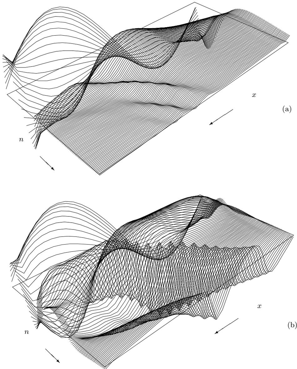
FIG. 4.1. The residual along the nozzle,  $x$ , plotted against the number of iterations,  $n$ , obtained using (a) nonreflective boundary conditions and (b) a well-posed but reflective boundary condition, pressure. The number of iterations shown is 100, and  $\nu = 0.97$  with  $N = 33$ .
