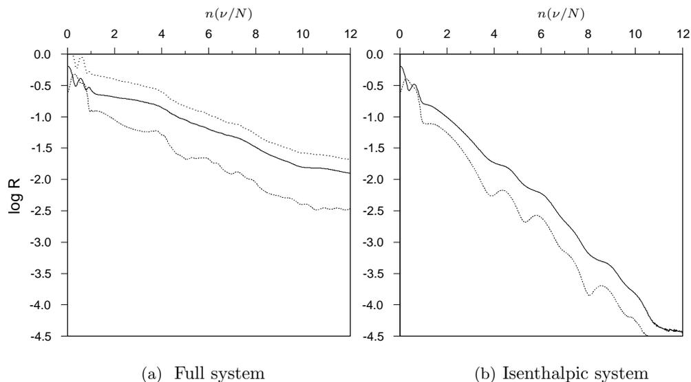
FIG. 4.2. Comparison of the convergence rates at  $N = 65$  with  $\nu = 0.97$  showing the residual of  $R(\rho)$ ,  $R(\rho u)$ , and  $R(\rho e)$  shown in solid, dashed, and dotted lines (for the full system only) and  $M_\infty = 0.4$ .
