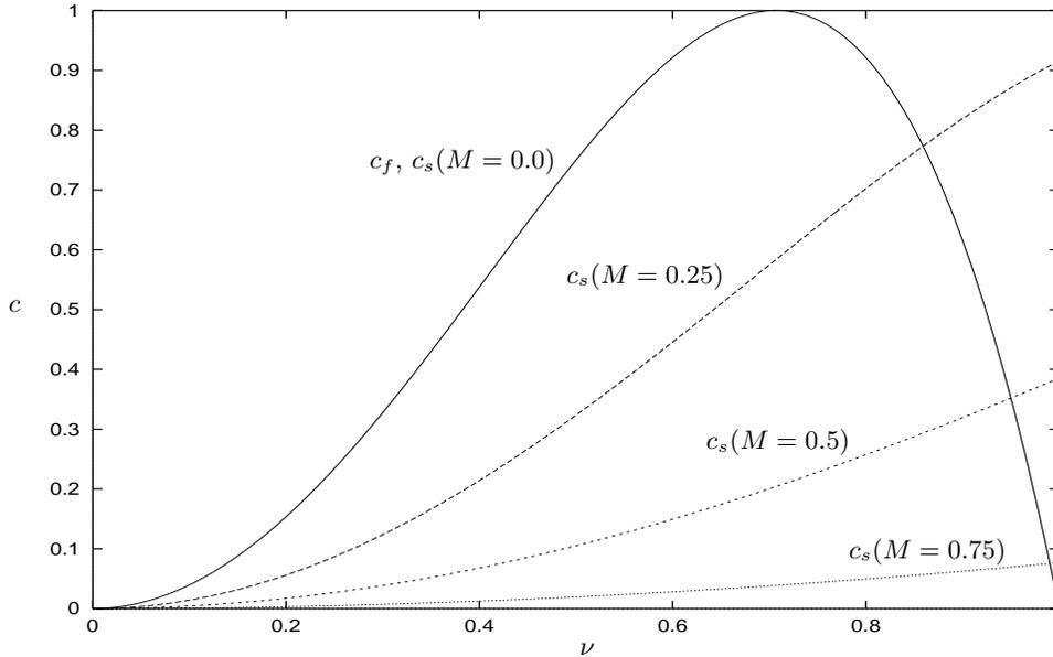
FIG. 3.1. Damping coefficient for LW as a function of Mach number for modes associated with the fast wave  $\nu_f$  and slow wave  $\nu_s$  for the isenthalpic system. If  $M = 0$ , the damping is exactly the same for both waves. As the Mach number increases the critical value of the CFL number at which the slow wave is damped better than the fast wave increases until at  $M = 1.0$ , at which point the slow wave is not damped at all.
