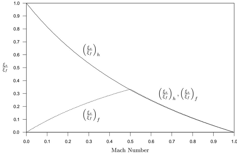
FIG. 3.2. Comparison of the eigenvalues of the full and *H*-systems, showing the slowest/fastest eigenvalue.
