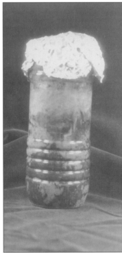
Figure 1. (b) Cover added to reduce evaporation from the column.
