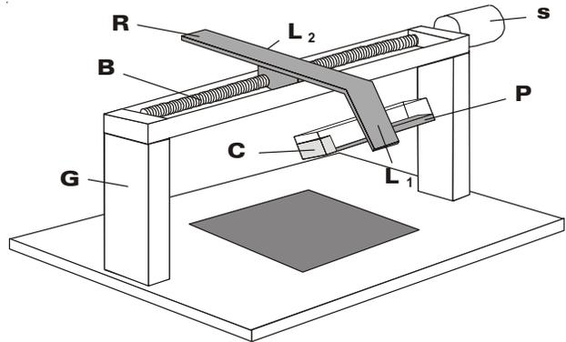
Figure 3. Sensor design used in this study. B = ball screw carriage; C = camera; G = gantry; L<sub>1</sub> = position 1; L<sub>2</sub> = position 2; P = projector; R = rail; S = stepper motor.
