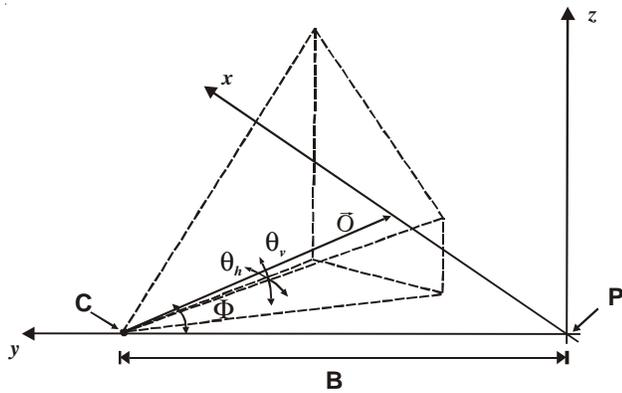
Figure 2. Geometric relationships among sensor elements that determine the level of spatial quantization for a given sensor design. B = baseline distance,  $\Phi$  = toe-in angle,  $\theta_h$  = horizontal angular field of view of the camera,  $\theta_v$  = vertical angular field of view of camera.
