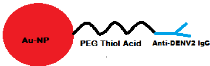
Figure 3. Proposed schematic of Bio-conjugation of anti-DENV2 IgG (HB46) to gold nanoparticles (AuNP). AuNPs are incubated with polyethylene glycol (PEG) and is bound via Au-Sulfur interaction. Purified HB46 IgG js then incubated with the AuNP-PEG via -COOH end binding to the thiol (S) acid. Estimates of approximately 100 IgGs can be bound to 1 AuNP ( Paul et al., 2014 ) 24 .
